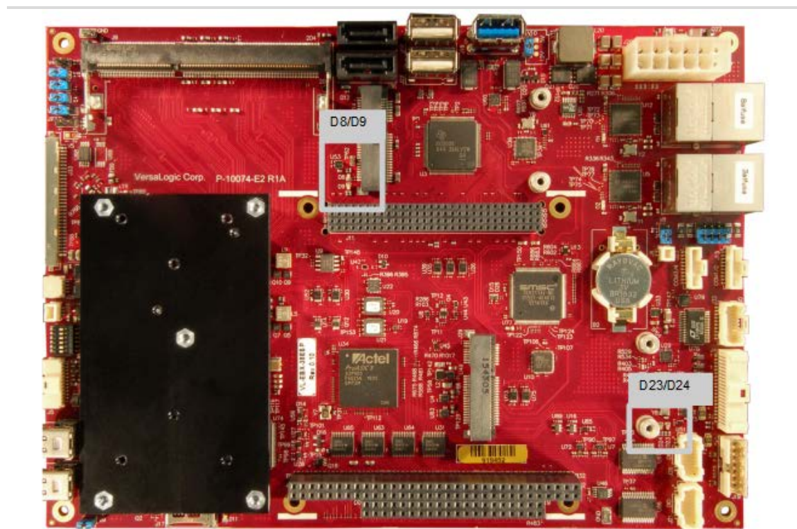
Figure 14. Location of PCIe Mini Card LEDs
