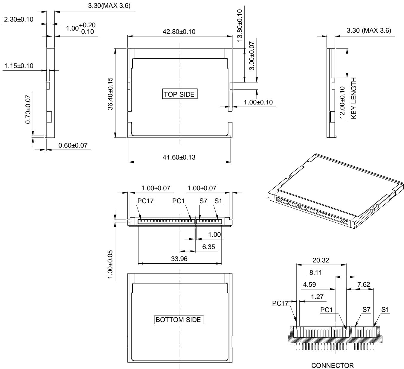
**Figure 2: Mechanical Dimensions**
