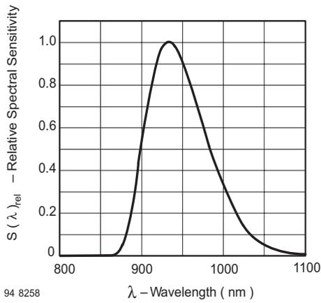
Figure 10. Relative Spectral Sensitivity vs. Wavelength
