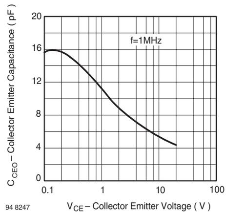
Figure 8. Collector Emitter Capacitance vs. Collector Emitter Voltage
