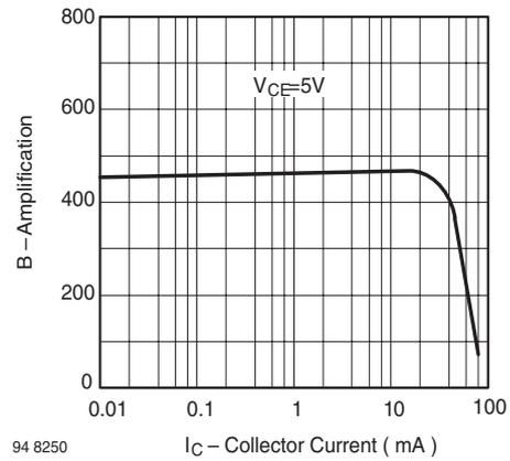
Figure 6. Amplification vs. Collector Current
