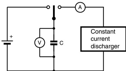
Fig. 4 - Test circuit for capacitance measurement
