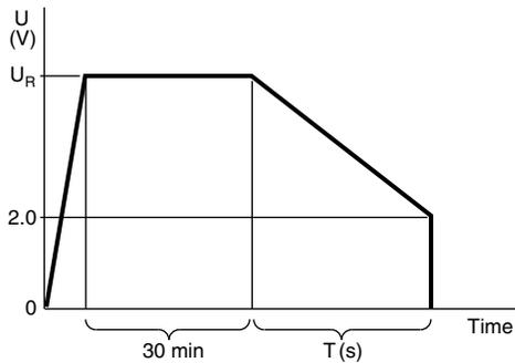
Fig. 3 - Voltage diagram for capacitance measurement
