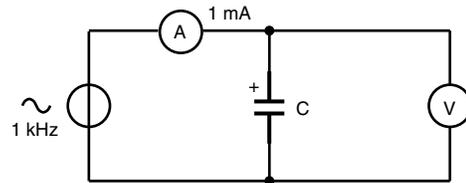
Fig. 5 - Test circuit for R<sub>I</sub> measurement
