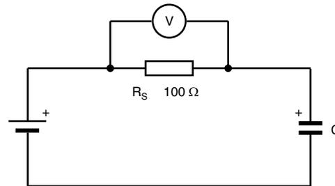
Fig. 6 - Test circuit for leakage current
