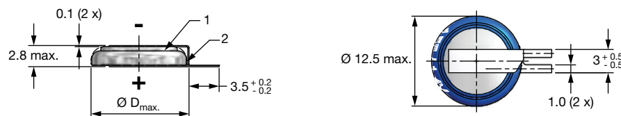
Fig. 6 - Form D2: Surface Mount Flat (single cell, keyed polarity)
