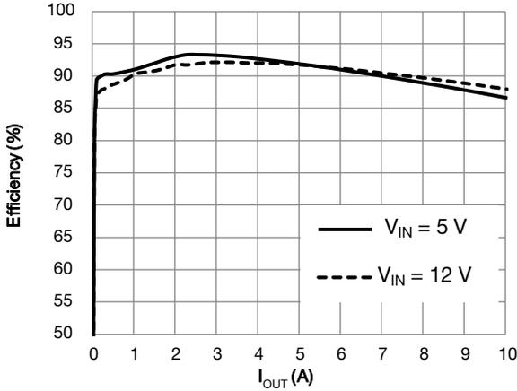
Fig. 1 - PSM Efficiency - V<sub>IN</sub> vs. Load (V<sub>DD</sub> = 3.3 V, V<sub>OUT</sub> = 1.5 V)
