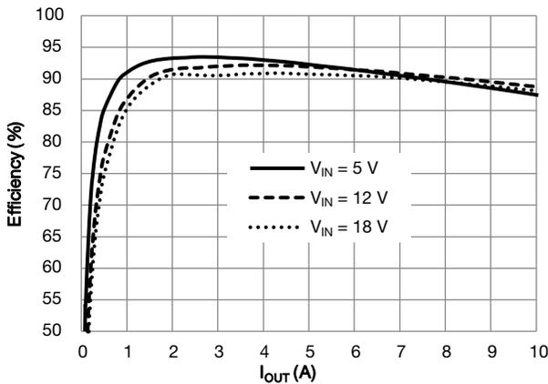
Fig. 3 - PSM Efficiency - V<sub>IN</sub> vs. Load (V<sub>DD</sub> = 5 V, V<sub>OUT</sub> = 1.5 V)
