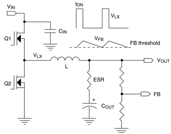
**Fig. 23 - PWM Control Method,  $V_{OUT}$  Ripple**
