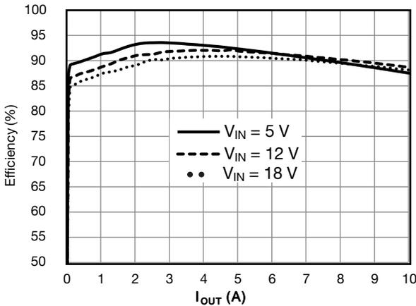
Fig. 2 - PSM Efficiency - V<sub>IN</sub> vs. Load (V<sub>DD</sub> = 5 V, V<sub>OUT</sub> = 1.5 V)
