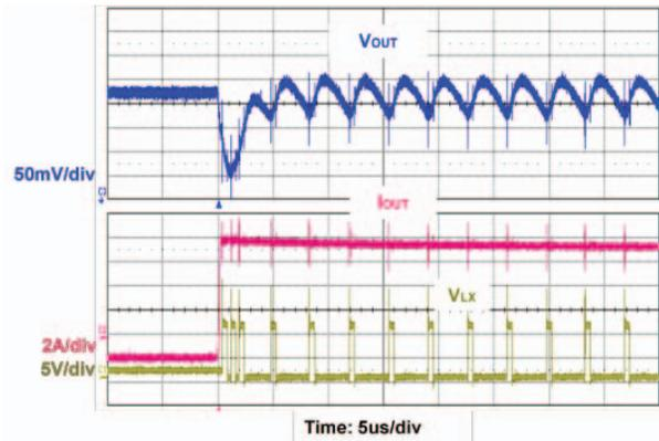
**Fig. 19 - Transient Response - PSM Rising ( $V_{DD} = 5\text{ V}$ ,  $V_{IN} = 12\text{ V}$ ,  $V_{OUT} = 1.5\text{ V}$ ,  $I_{OUT} = 0.5\text{ A}$  to  $8.5\text{ A}$ ,  $di/dt = 1\text{ A}/\mu\text{s}$ )**
