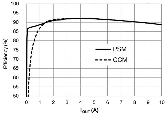
Fig. 5 - Efficiency - PSM vs. CCM (V<sub>DD</sub> = 5 V, V<sub>OUT</sub> = 1.5 V, V<sub>IN</sub> = 12 V)
