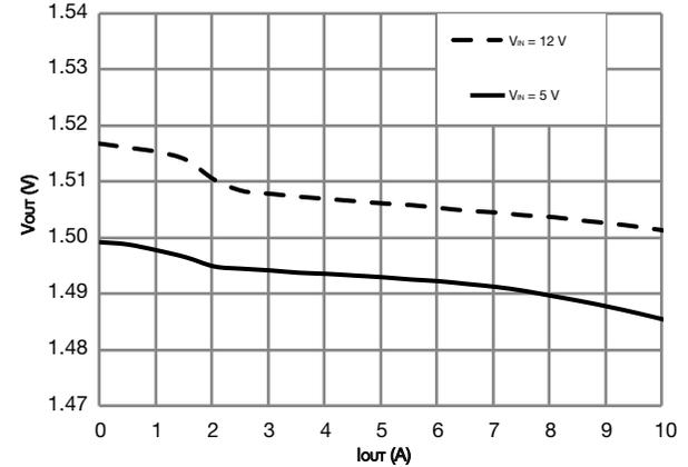
Fig. 11 - Load Regulation - PSM (V<sub>DD</sub> = 3.3 V, V<sub>OUT</sub> = 1.5 V)
