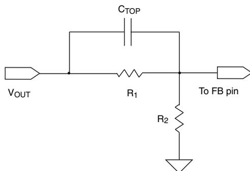
**Fig. 35 - Capacitor Coupling to FB Pin**
