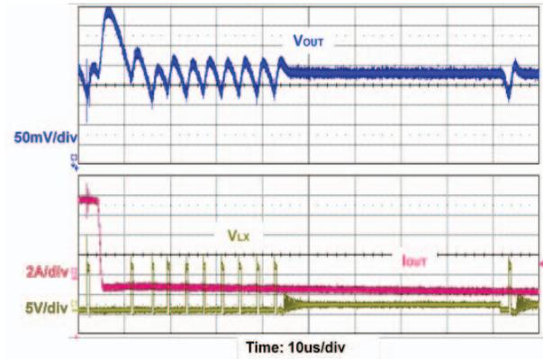
**Fig. 21 - Transient Response - PSM Falling ( $V_{DD} = 5\text{ V}$ ,  $V_{IN} = 12\text{ V}$ ,  $V_{OUT} = 1.5\text{ V}$ ,  $I_{OUT} = 8.5\text{ A}$  to  $0.5\text{ A}$ ,  $di/dt = 1\text{ A}/\mu\text{s}$ )**
