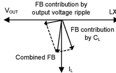
**Fig. 39 - FB Voltage in Phasor Diagram**
