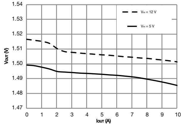
Fig. 10 - Load Regulation - FCM (V<sub>DD</sub> = 3.3 V, V<sub>OUT</sub> = 1.5 V)
