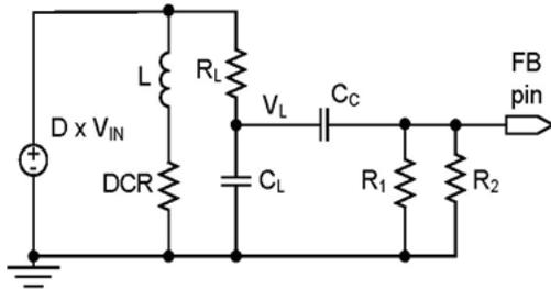
**Fig. 37 - FB Voltage by  $C_L$  Voltage**
