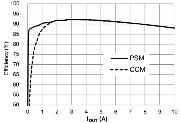
Fig. 4 - Efficiency - PSM vs. CCM (V<sub>DD</sub> = 3.3 V, V<sub>OUT</sub> = 1.5 V, V<sub>IN</sub> = 12 V)
