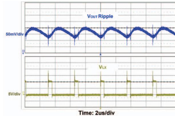
**Fig. 18 - Forced Continuous Mode - SiC402ACD**
