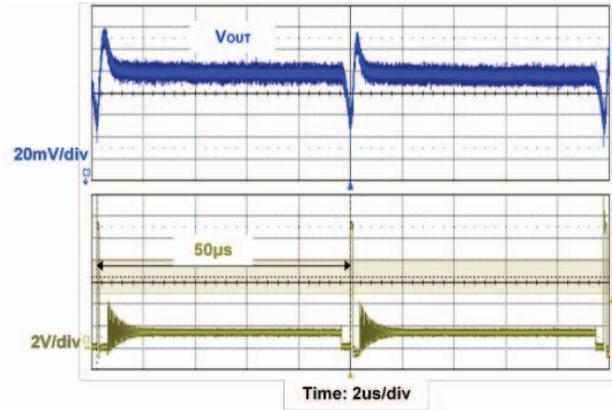
**Fig. 17 - Ultra-sonic PSM - SiC402ACD**
