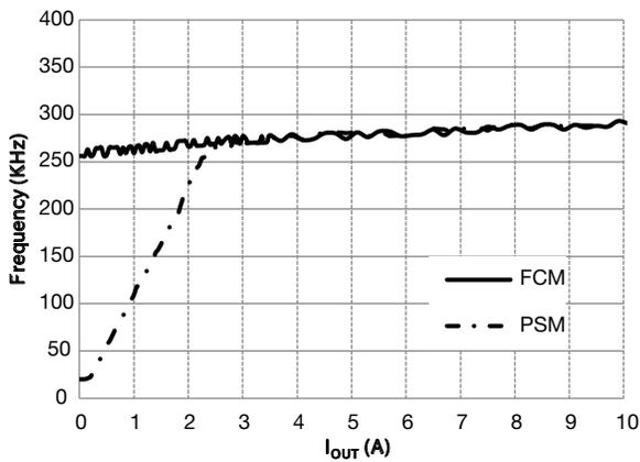
Fig. 9 - Switching Frequency - PSM vs. FCM (V<sub>DD</sub> = 5 V, V<sub>OUT</sub> = 1.5 V, V<sub>IN</sub> = 12 V)
