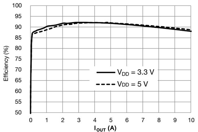
Fig. 6 - PSM Efficiency - V<sub>DD</sub> 3.3 V vs. 5 V (V<sub>OUT</sub> = 1.5 V, V<sub>IN</sub> = 12 V)
