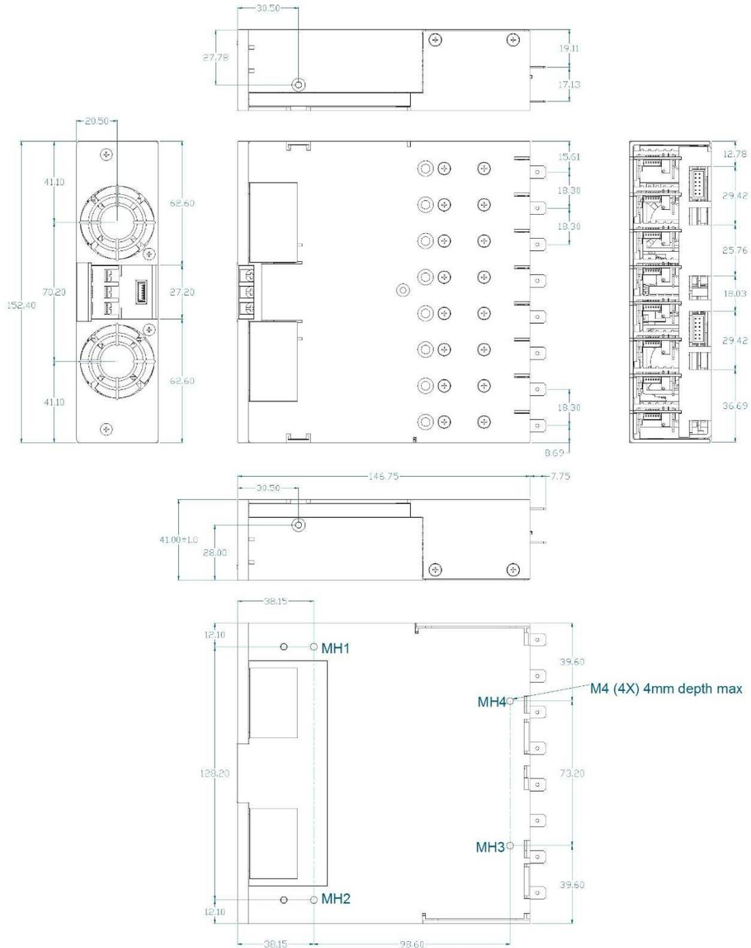
TOLERANCES unless otherwise stated - All dimensions in mm and according to DIN 2768-1/-2 CLASS C
