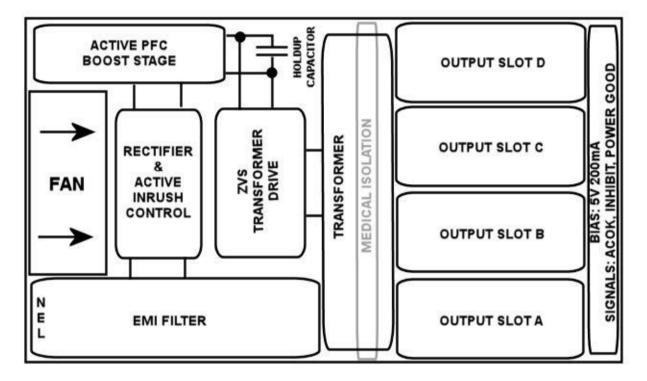
The *input module* is responsible for receiving the AC mains line voltage and converting it to an appropriate DC voltage whilst providing protection from AC line disturbances and preventing excessive EMI emissions and current harmonics. The integrated EMI filter attenuates high frequency current emissions to levels below EN55022 class B. It also provides single pole fusing in the live conductor and protection from line disturbances as outlined in EN61000.
