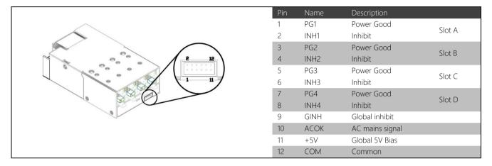
All of the signals are referenced to the bias supply common rail (COM) and external control and/or monitoring circuits can be easily powered and interfaced to the PSU through this connector. The entire signals circuit is fully medically isolated and can be considered a SELV output. The table below lists the isolation voltages.
