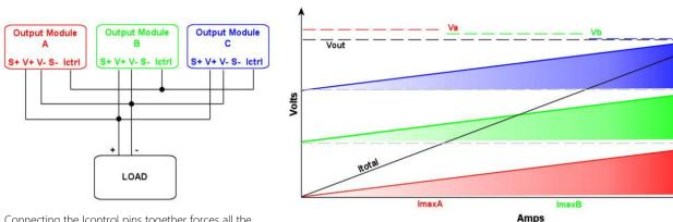
Connecting the Icontrol pins together forces all the outputs to deliver the same current, ensuring that
