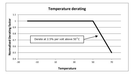
Depending on the application conditions, one or both of the deratings may apply. Where both apply, the derating factors given above can be multiplied together to obtain the total derating factor.
