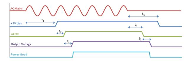
Typical timing values:  $t_1 \phi$  300 ms,  $t_2 \phi$  50 ms,  $t_3 \phi$  25 ms,  $t_4 \phi$  15 ms,  $t_5 = 5$  ms (minimum),  $t_6 \phi$  100 ms
