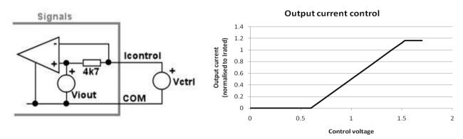
In the diagram above, Vi\_out is an internal voltage source that is proportional to the internal inductor current and approximates the equation,
