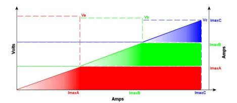
In this mode the highest adjusted output module will supply all of the load current until it's current limit is
