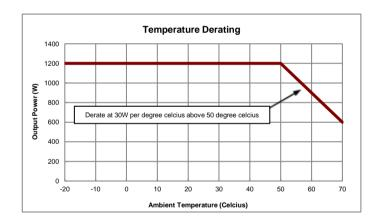
Depending on the application conditions, one or both of the de-ratings may apply. Where both apply, calculate each de-rating in turn and fill the result from the first calculation into the second calculation.
