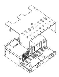
Insert the modules as the configuration requires – 1 OP1 module into Slot A, Slot B, Slot C and Slot D; 1 OP2 module into Slot E; 1 OP3 module in Slot E and 1 OP4 module into Slot F.
