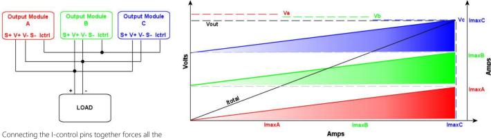
Connecting the I-control pins together forces all the outputs to deliver the same current, ensuring that
