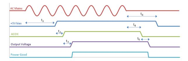
Typical timing values at 25°C:  $t_1 \varphi$  2000 ms,  $t_2 \varphi$  50 ms,  $t_3 \varphi$ 25 ms,  $t_4 \varphi$  15 ms,  $t_5 = 5$  ms (minimum),  $t_6 \varphi$  100 ms
