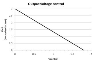
The output voltage can be controlled from 0% to 300% of the preset voltage using this control method. However, care must be taken to ensure the output voltage does not exceed the OVP level, as this is considered a safety hazzard and will latch the entire unit off. To determine the level of control voltage that will trigger OVP, insert Vovp into the equation above.
