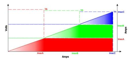
In this mode the highest adjusted output module will supply all of the load current until it's current limit is
