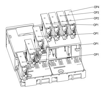
The Blanking Plate is inserted directly into the lid as shown below and should be done before putting the chassis lid back onto the chassis base.
