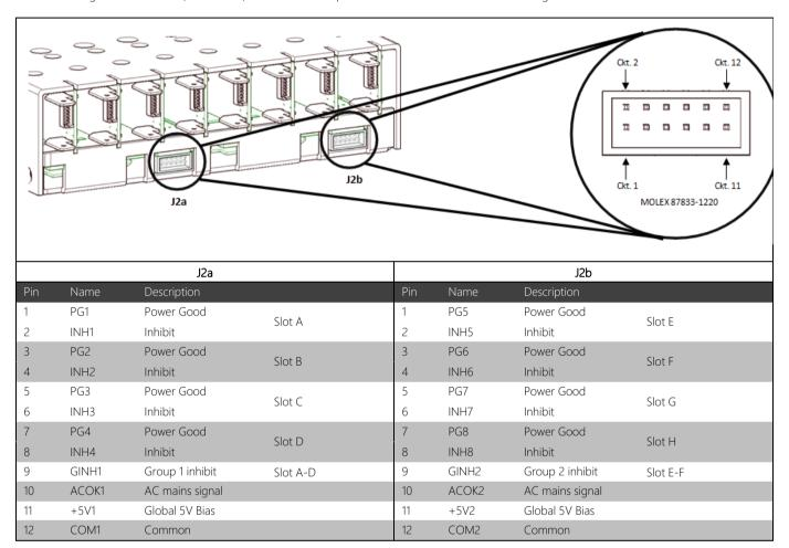
All of the signals are referenced to the relevant group bias supply common rail (COM) and external control and/or monitoring circuits can be easily powered and interfaced to the PSU through these connectors. Both entire signals circuits are fully medically isolated and can be considered a SELV output. The table below lists the isolation voltages.
