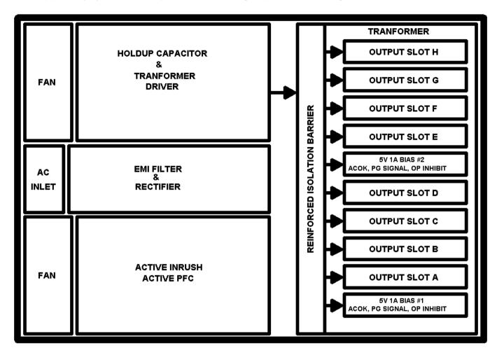
The *input module* is responsible for receiving the AC mains line voltage and converting it to an appropriate DC voltage whilst providing protection from AC line disturbances and preventing excessive EMI emissions and current harmonics. The integrated EMI filter attenuates high frequency current emissions to levels below EN55022 class B. It also provides single pole fusing in the live conductor and protection from line disturbances as outlined in EN61000.
