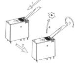
Easy to use: test lever for mechanical operation of the contacts
