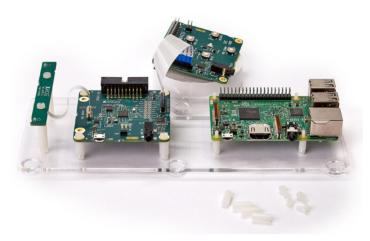
3. Screw the longer spacers into place on top of the RPi and then push the Pi HAT onto the RPi.
