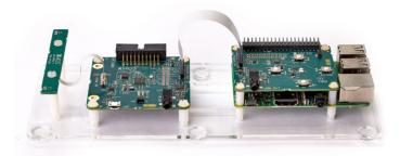
5. Turn the kit over and slide the SD card into the Pi through the hole in the plastic kit stand. Make sure that NOOBS is installed before you add the SD Card to the kit.
