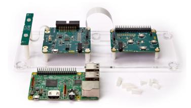
2. Fix the Raspberry Pi to the plastic stand using the shorter plastic spacers to support the RPi.
