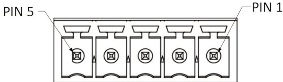
To use a potentiometer as the control source connect one end of the potentiometer to the 3.0 Volt Reference, the other end to Ground and the wiper to the control Input. The potentiometer should be in the range of 1K to 10K ohms. Set the power supply to run from a 3 volt analog input on voltage or current or both.
