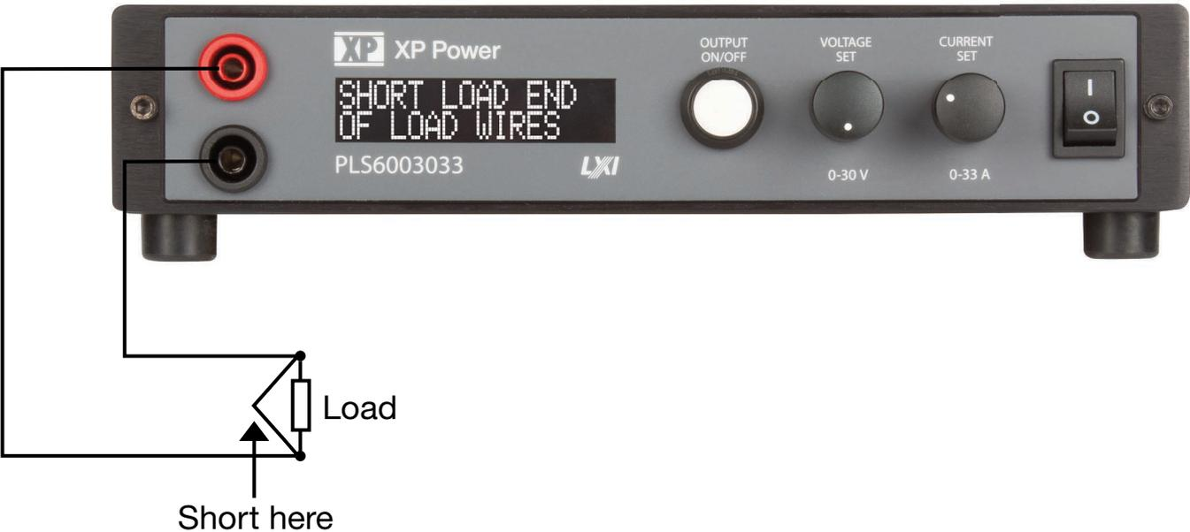
It is important that a good short with heavy wire is made as failure to do this will result in a poor remote sense calibration.
