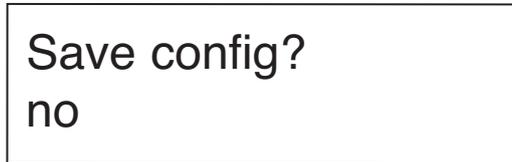
When the desired option is displayed press the output on/off button. Selecting YES will save any Setup changes to non-volatile memory and they will be retained even when primary power is cycled. Selecting NO will not save Setup changes to non-volatile memory and they will be in effect only until the unit is turned off.
