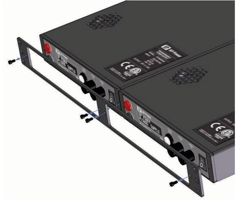
5) If a second power supply is to be mounted on the rack mount kit begin with Step 2 above. If a blank panel is to be mounted in place of a second power supply use provided panel and screws. See figure below.
