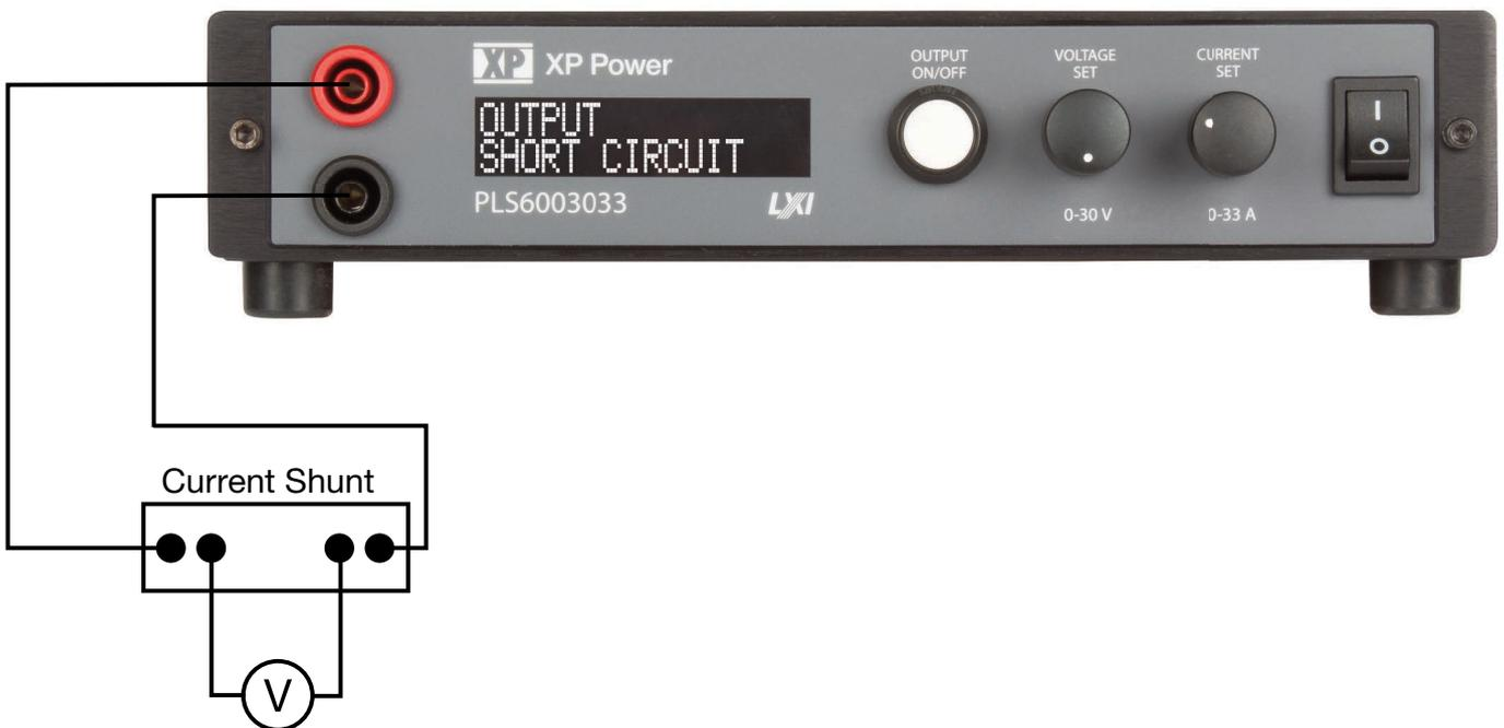
When the power supply is configured as in the figure on previous page, press the output on/off button. The following screen will now appear:
