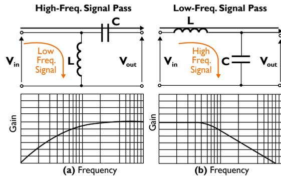
Filtering functions of capacitor coupled with inductor
