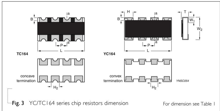
Fig. 3 YC/TC164 series chip resistors dimension
