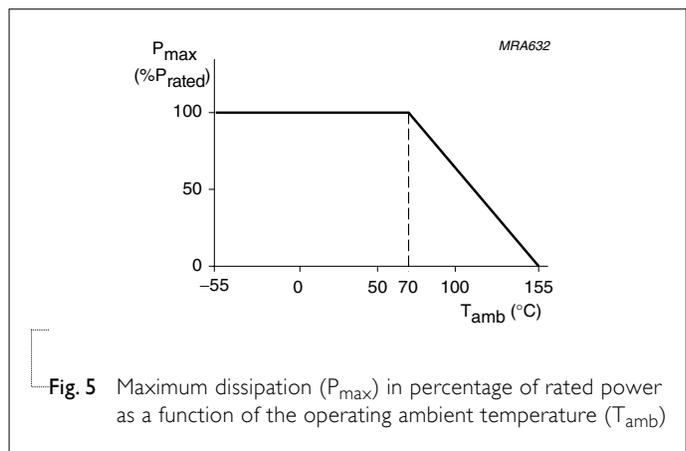
Fig. 5 Maximum dissipation (P<sub>max</sub>) in percentage of rated power as a function of the operating ambient temperature (T<sub>amb</sub>)
