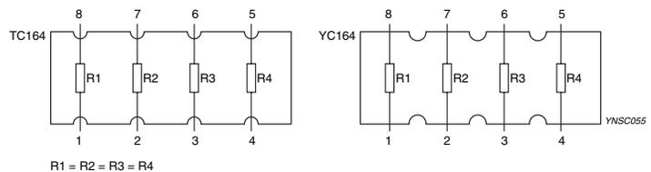
Fig. 4 Equivalent circuit diagram
