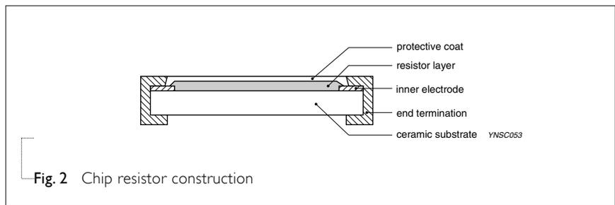
Fig. 2 Chip resistor construction
