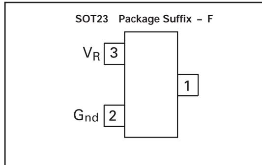
Top view - Pin 1 floating or connected to pin 2
