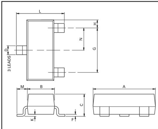
Controlling dimensions are in millimeters.
