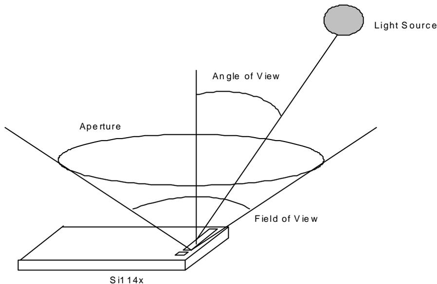
**Figure 12. Aperture, Field of View and View Angle**
