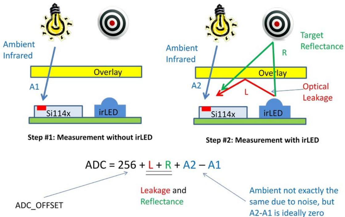
Figure 23. Proximity Measurement Concept
