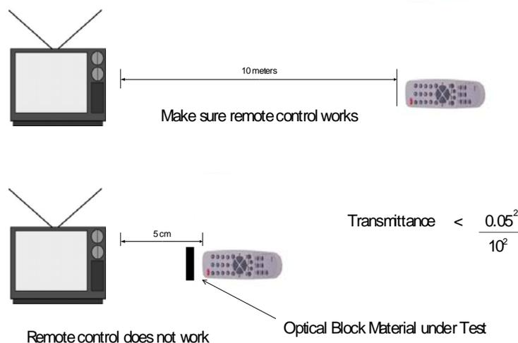
**Figure 6. Infrared Opacity Test**
