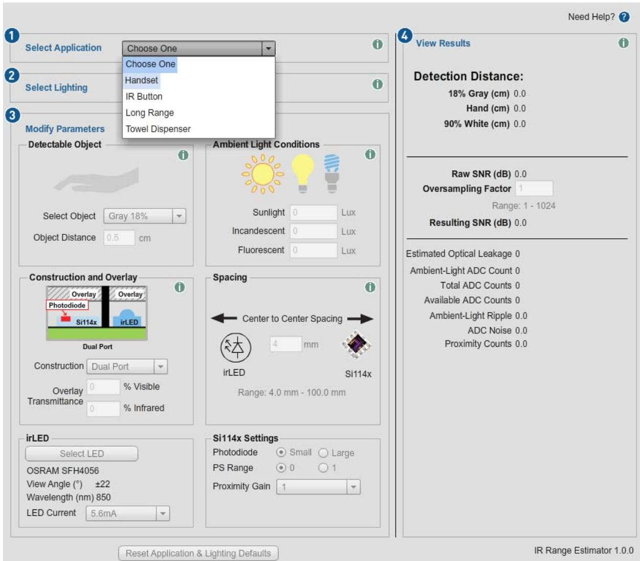
Figure 31. IR Range Estimator Application Selection
