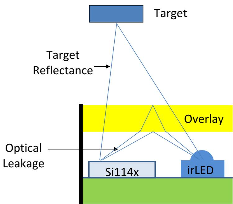
**Figure 4. Optical Leakage**
