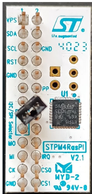
Figure 6. Use of the I2C/SPI jumper for the I2C interface selection
