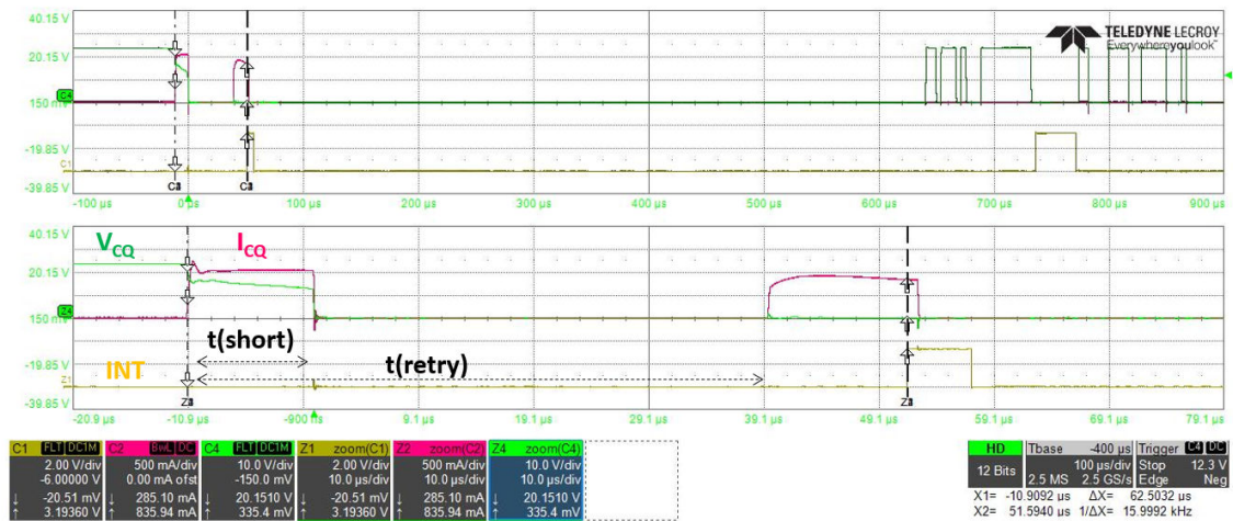
Figure 4. Example of wake-up sequence timing ( V_{CQ} = green plot; I_{CQ} = red plot; V_{INT} = Yellow)
