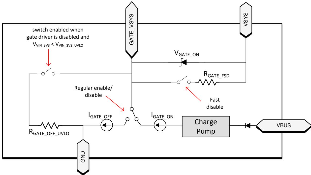
**Figure 9-17. Details of the VSYS Gate Driver**
