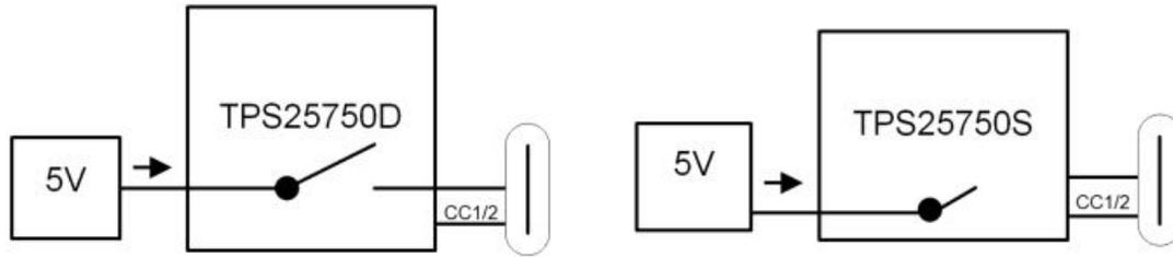
Figure 10-5. Power Source Only Configuration
