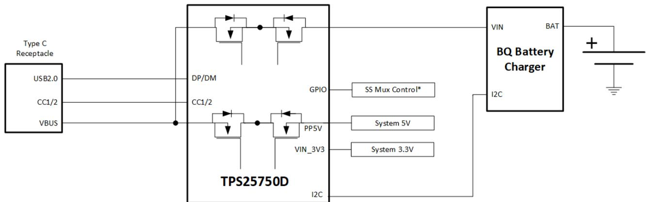
Figure 10-6. Power Only Battery Charger Application Block Diagram
