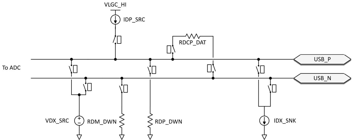
Figure 9-23. BC1.2 Hardware Components (External for DRP)
