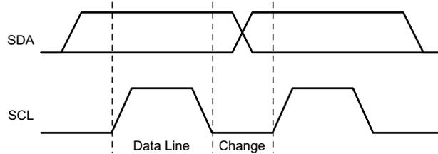
**Figure 9-27. I<sup>2</sup>C Bit Transfer**
