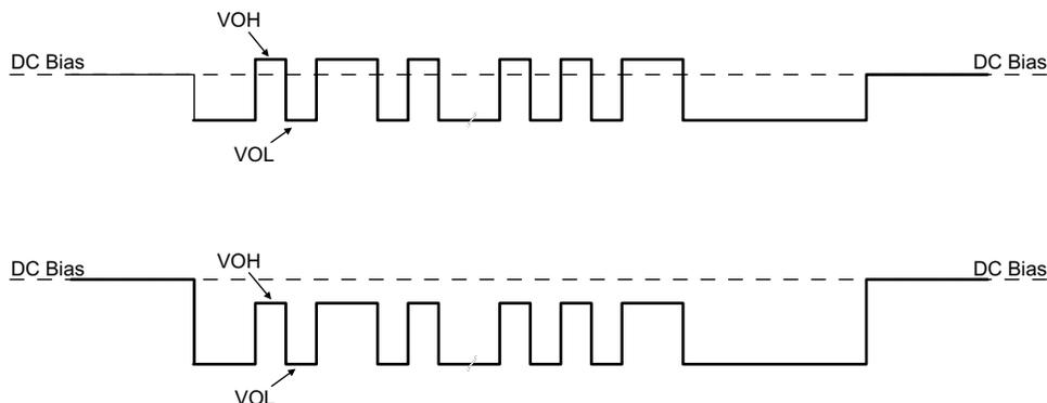
**Figure 9-8. TX Driver Transmission with DC Bias**
