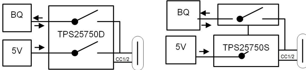
**Figure 10-2. Power Source and Sink configuration with the Battery Charger (BQ)**
