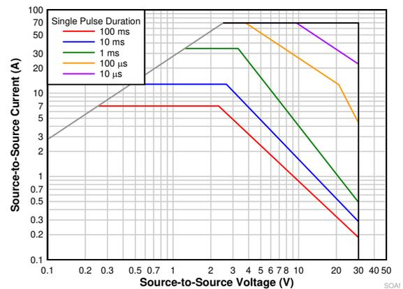
Figure 7-6. Safe-Operating-Area (SOA) of PPHV for TPS25750D
