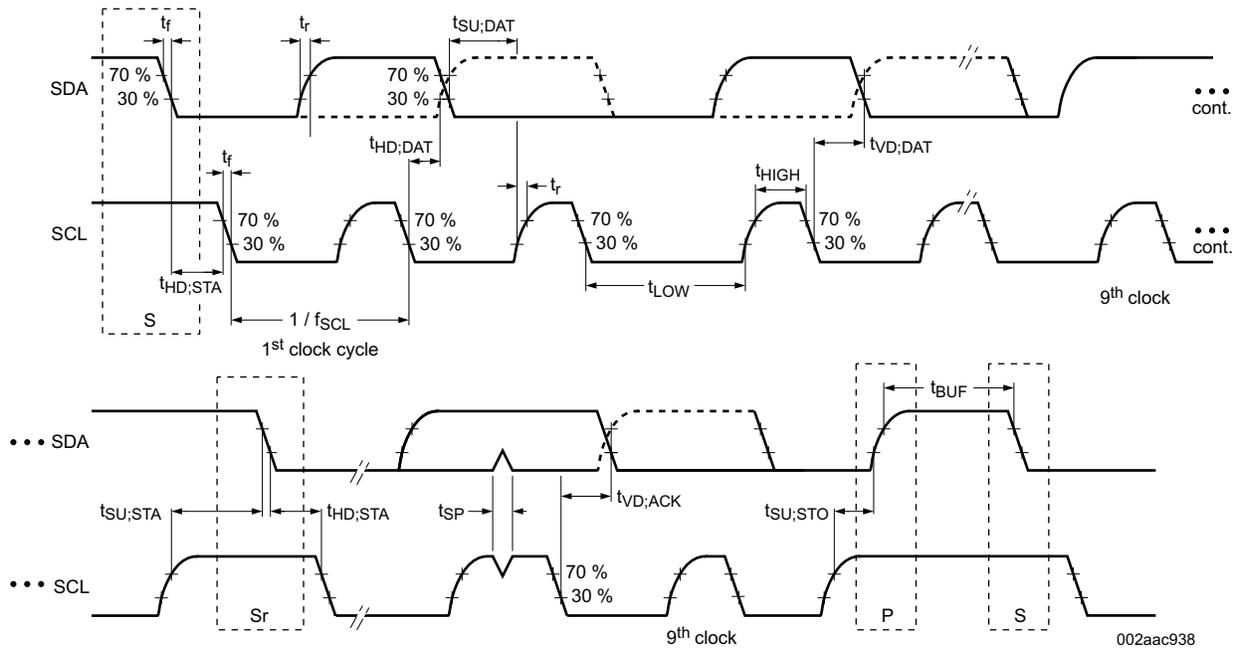
Figure 8-1. I<sup>2</sup>C Slave Interface Timing
