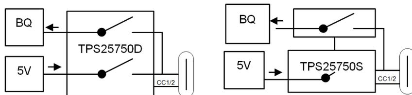
**Figure 10-3. Power Source and Sink configuration with 5V DC and Battery Charger (BQ)**
