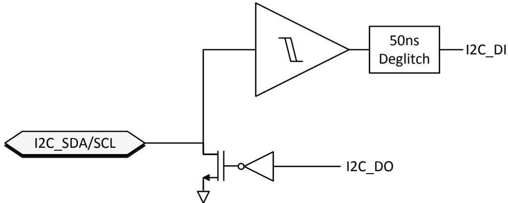
Figure 9-24. I<sup>2</sup>C Buffer
