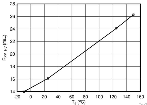
Figure 7-5. R<sub>PPHV</sub> vs. Temperature for TPS25750D
