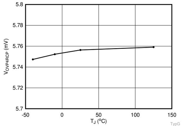
Figure 7-4. V<sub>OVP4RCP</sub> (Setting 2) vs. Temperature
