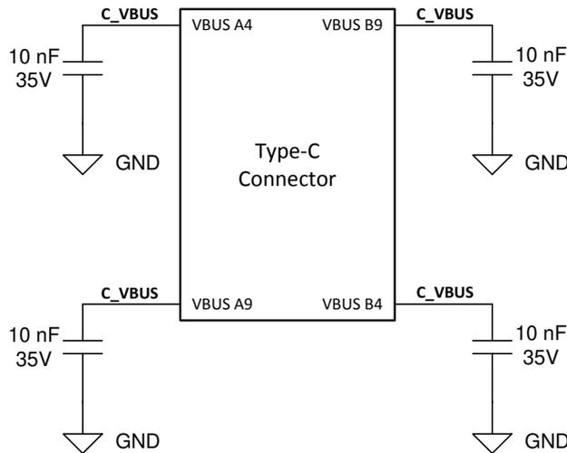
**Figure 10-7. Type-C Connector VBUS Capacitors**
