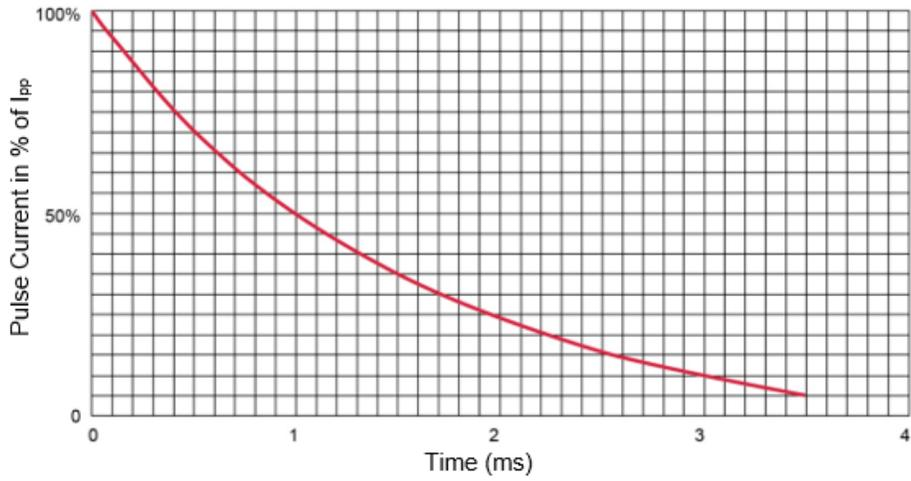
Figure 3-4. Current Impulse Waveform ( $I_{PP} = 8 \mu\text{s}$ )
