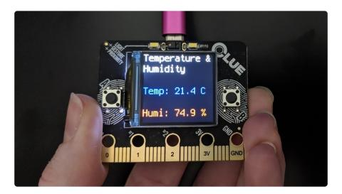
Note: The temperature will read higher than ambient temperature because of the backlight on the CLUE display.
