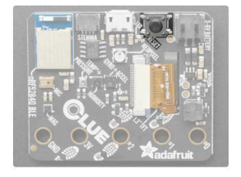
**Reset button** - This button resets the board. Press once to reset. Quickly press twice to enter the bootloader.
