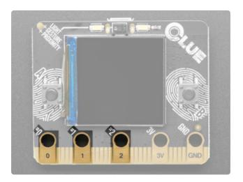
Pads 0, 1 and 2 - These pads are used for connecting external sensors etc, typically using alligator clips. They also work as inputs using capacitive touch. In CircuitPython they are board.D0, board.D1, and board.D2. In Arduino, they are D0, D1 and D2.
