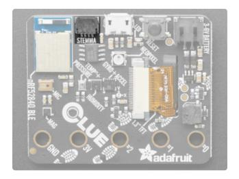
Qwiic / STEMMA QT connector - Use to add more sensors, motor controllers, or displays over I2C. You can plug in GROVE I2C sensors by using an adapter cable (http://adafru.it/4424).
