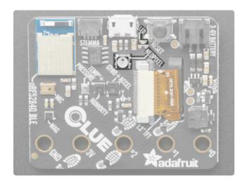
NeoPixel - The addressable RGB NeoPixel LED is used as a status LED by the bootloader and CircuitPython, but is also controllable using code. Control it using board.NEOPIXEL in CircuitPython and D18 in Arduino.
