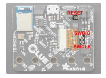
On the bottom of the board are three pads, one near the reset button, and two to the right of the display cable. The pad near the reset button is reset. Of the two pads near the display cable, the top is SWDIO and on the bottom is SWCLK. On the off chance you want to reprogram your CLUE or debug it using a debug/ programmer, you will need to solder/ connect to these pads.
