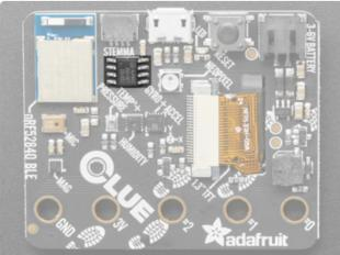
Nordic nRF52840 Bluetooth LE processor - 1 MB of Flash, 256KB RAM, 64 MHz Cortex M4 processor.
