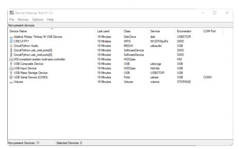
Select all the devices you want to remove, and then press Delete. It is usually safe just to select everything. Any device that is removed will get a fresh install when you plug it in. Using the Device Cleanup Tool also discards all the COM port assignments for the unplugged boards. If you have used many Arduino and CircuitPython boards,
