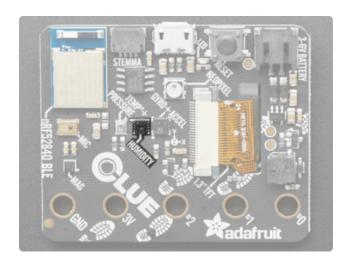
Humidity: SHT30 - This sensor has an excellent  $\pm 2\%$  relative humidity and  $\pm 0.5^{\circ}$ C accuracy for most uses. Sensor is I2C on standard pins on address 0x44.
