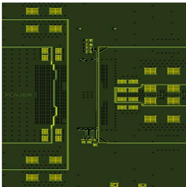
**Figure 18: Backside Decoupling**
