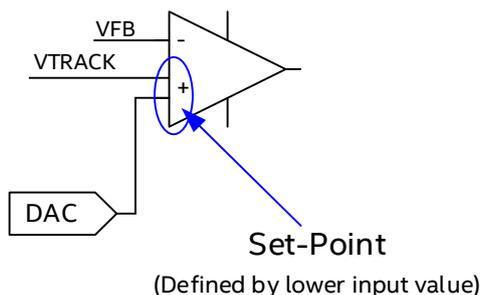
**Figure 9: VTRACK Circuitry**
