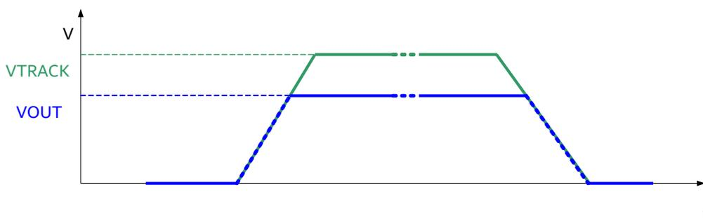
**Figure 11: Simultaneous Sequencing Using VTRACK**
