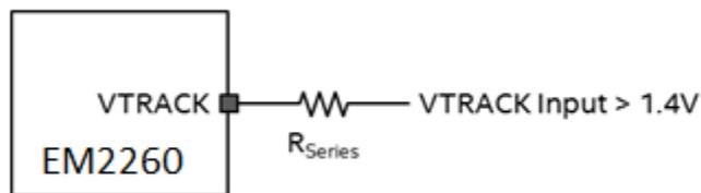
**Figure 13: VTRACK Sense Circuitry (Input > 1.4V)**
