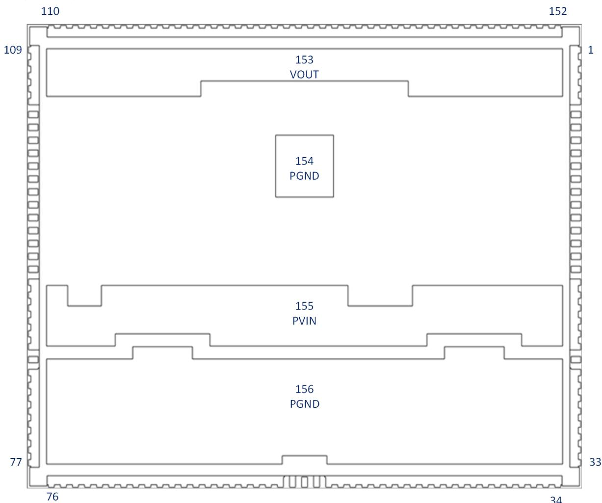
Figure 2: Pin Out Diagram Bottom side
