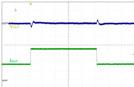
$V_{IN} = 12V, V_{OUT} = 0.9V, 40 \mu s/div$
