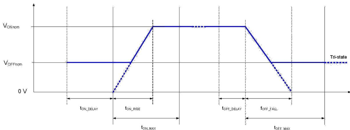
Figure 7: Power Sequencing with Non-Zero Off Voltage
