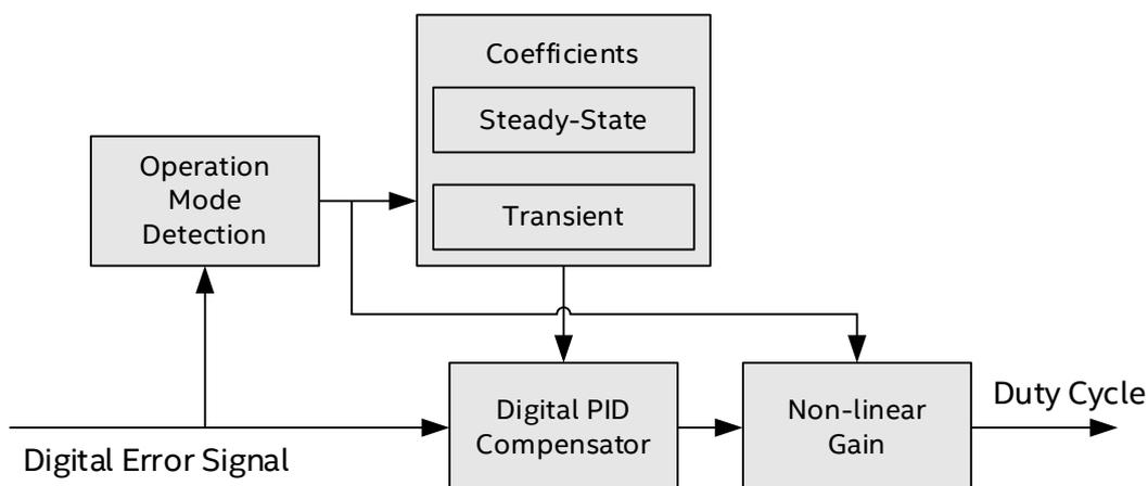
**Figure 4: Simplified Block Diagram of The Digital Compensation**
