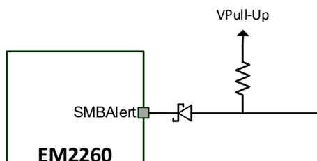
Figure 6: SMBAAlert Pin Low Voltage Pull-up Option
