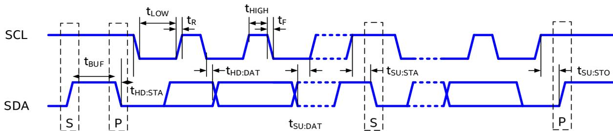
Figure 14: PMBus Timing Diagram
