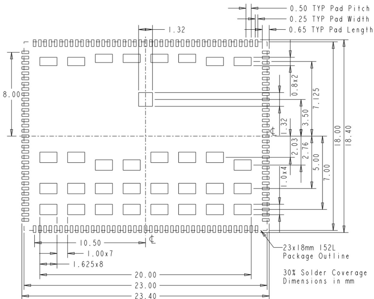
Figure 24: 30% Solder Stencil Aperture Dimensions
