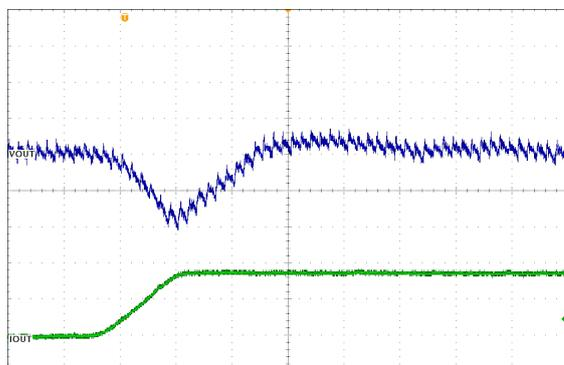
$V_{IN} = 12V, V_{OUT} = 0.9V, 2 \mu s/div$
