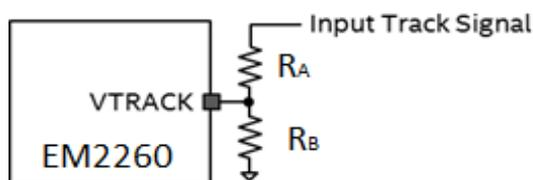
**Figure 12: VTRACK Sense Circuitry with Resistor Divider**
