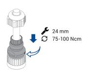
Screw the connector body to the contact holder.
