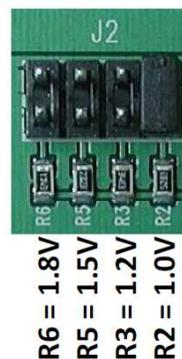
**CAUTION:** the VOUT jumper settings can only be changed when the device is off. Failure to follow this guideline may result in damage to the part.
