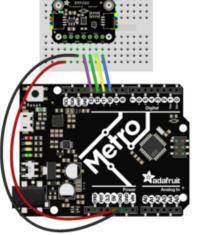
Connect **Vin** to the power supply, 3V or 5V is fine. Use the same voltage that the microcontroller logic is based off of. For most Arduinos, that is 5V Connect **GND** to common power/data
