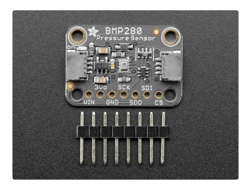
The BMP280 is the next-generation of sensors from Bosch, and is the upgrade to the BMP085/BMP180/BMP183 - with a low altitude noise of 0.25m and the same fast conversion time. It has the same specifications, but can use either I2C or SPI. For simple easy wiring, go with I2C. If you want to connect a bunch of sensors without worrying about I2C address collisions, go with SPI.
