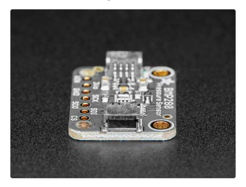
Nice sensor right? So we made it easy for you to get right into your next project. The surface-mount sensor is soldered onto a custom made PCB in the STEMMA QT form factor (https://adafru.it/LBQ), making them easy to interface with. The STEMMA QT connectors (https://adafru.it/JqB) on either side are compatible with the SparkFun Qwiic (https://adafru.it/Fpw) I2C connectors. This allows you to make solderless connections between your development board and the BMP280 or to chain it with a
