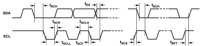
Figure 5. I<sup>2</sup>C Port Timing
