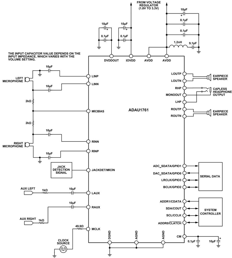
Figure 26. System Block Diagram
