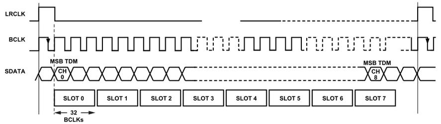
Figure 62. TDM 8 Mode with Pulse Word Clock
