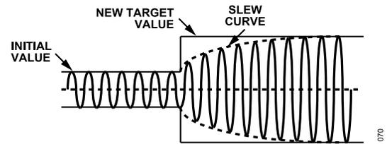
Figure 70. Example of Volume Slew
