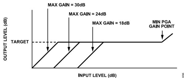
Figure 39. Effect of Varying the Maximum Gain Parameter
