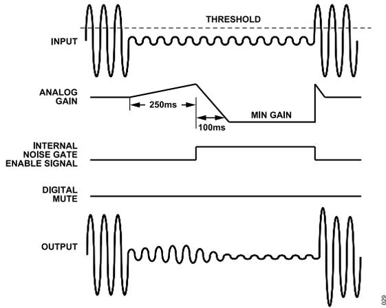
Figure 42. Noise Gate Mode 2 (Analog Fade)
