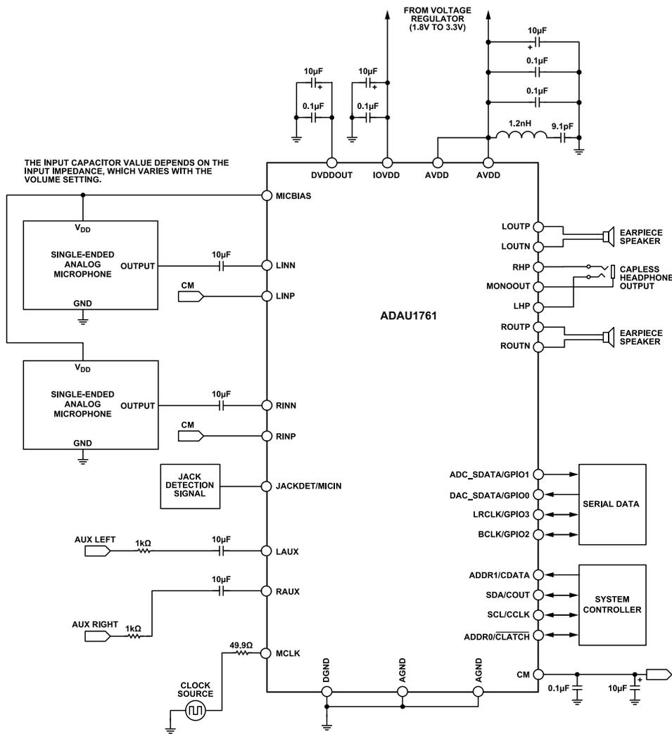
Figure 27. System Block Diagram with Analog Microphones
