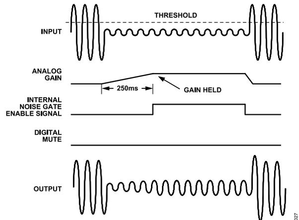
Figure 40. Noise Gate Mode 0 (PGA Gain Hold)
