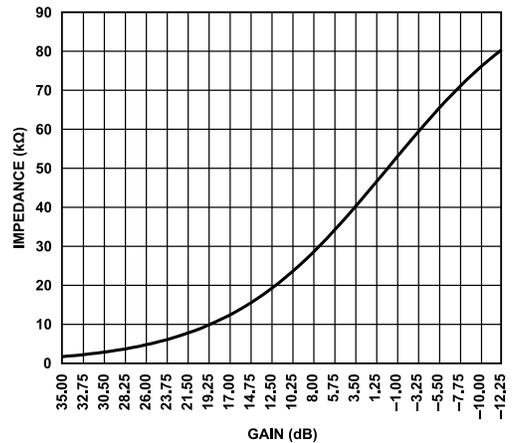
Figure 25. Input Impedance vs. Gain for Analog Inputs
