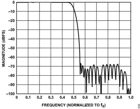
Figure 20. DAC Interpolation Filter, 128× Oversampling, Normalized to  $f_s$
