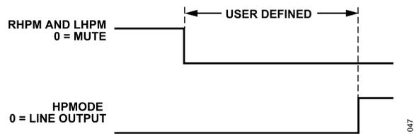
Figure 47. Headphone Output Power-Down Timing
