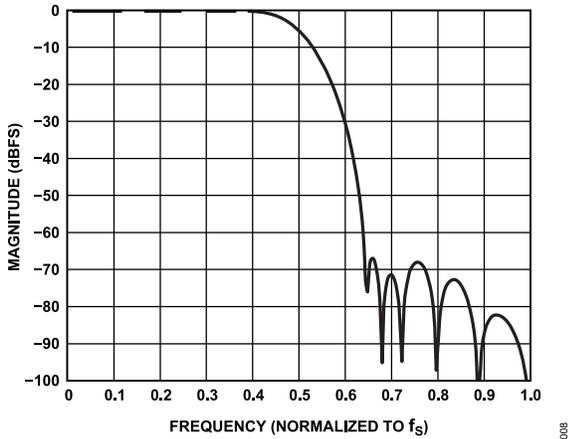
Figure 10. ADC Decimation Filter, 64× Oversampling, Normalized to  $f_s$
