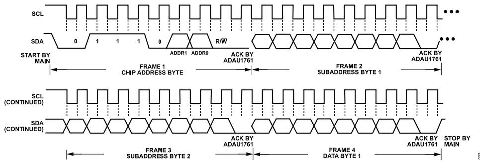
Figure 49. I<sup>2</sup>C Write to ADAU1761 Clocking
