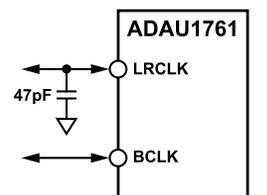
Figure 57. LRCLK Capacitor Alignment, TDM Pulse Mode
