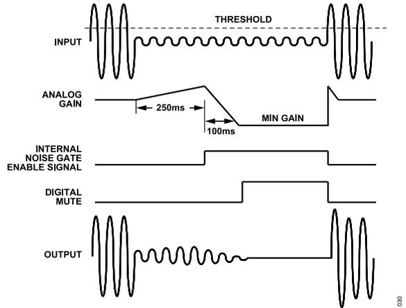
Figure 43. Noise Gate Mode 3 (Analog Fade/Digital Mute)
