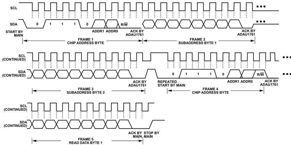
Figure 50. I<sup>2</sup>C Read from ADAU1761 Clocking
