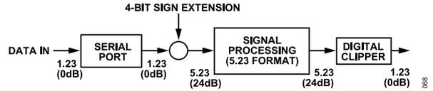
Figure 68. Numeric Precision and Clipping Structure
