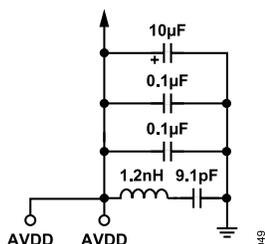
Figure 64. GSM Filter on the Analog Supply Pins
