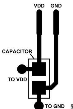
Figure 63. Recommended Power Supply Bypass Capacitor Layout
