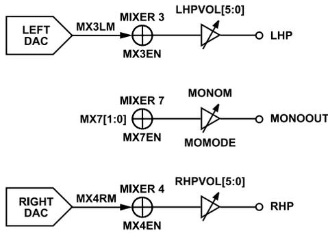
Figure 45. Capless Headphone Configuration Diagram
