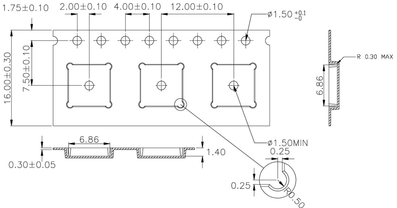
Sprocket hole pitch cumulative tolerance  $\pm 0.20$ .
