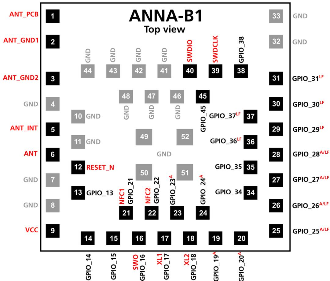
A = Analog function capable pin    LF = Low Frequency, low drive I/O only
