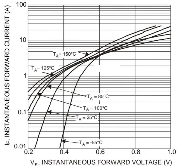
Fig. 2 Typ. Forward Characteristics - B350AQ thru B360AQ
