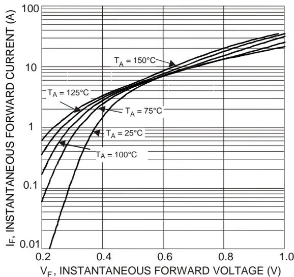
Fig. 1 Typical Forward Characteristics - B320AQ thru B340AQ
