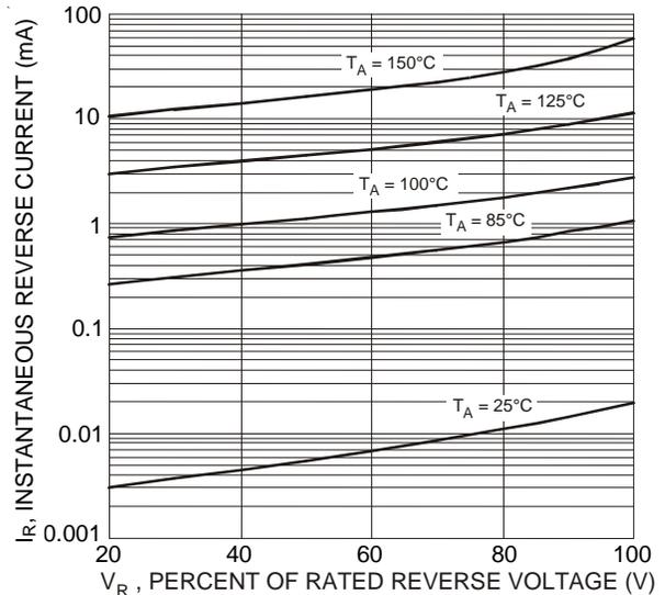
Fig. 4 Typical Reverse Characteristics, B350AQ thru B360AQ
