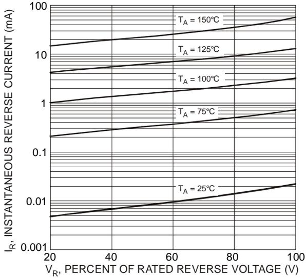
Fig. 3 Typical Reverse Characteristics, B320AQ thru B340AQ
