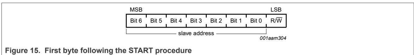
Figure 15. First byte following the START procedure
