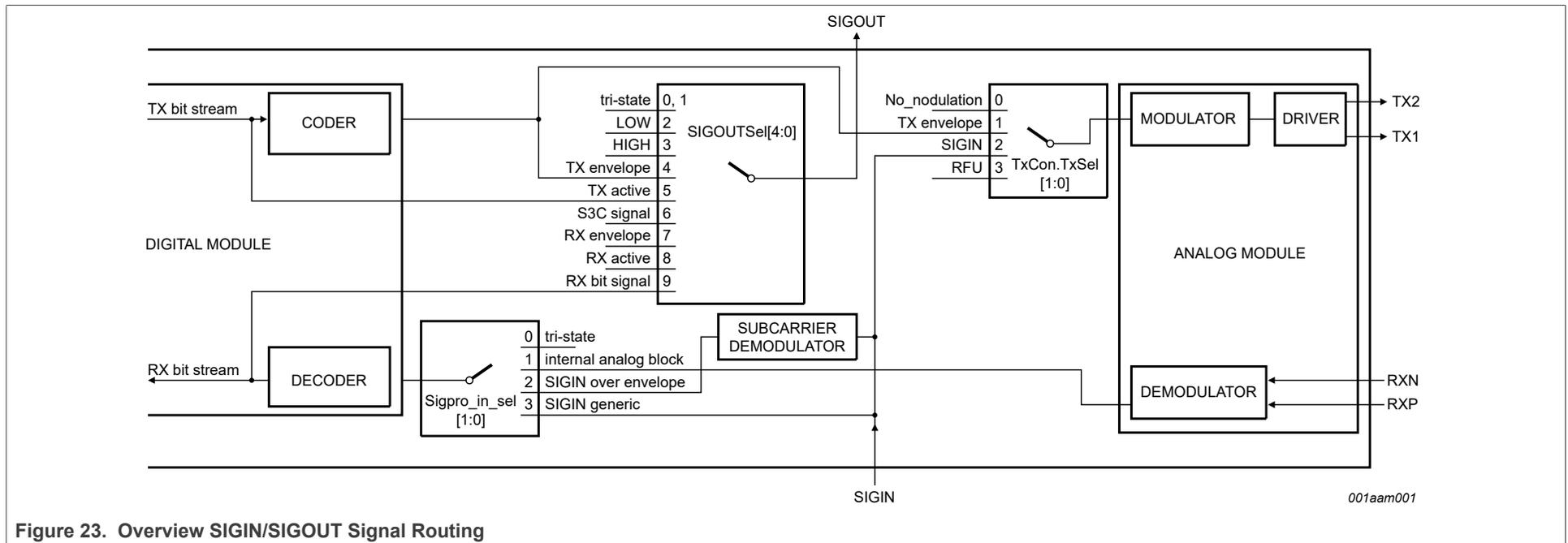
Figure 23. Overview SIGIN/SIGOUT Signal Routing
