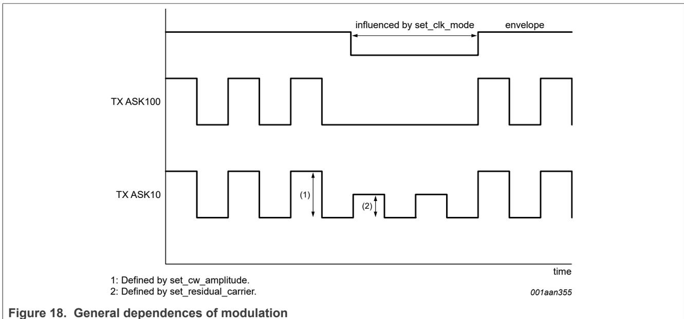
Note: When changing the continuous carrier amplitude, the residual carrier amplitude also changes, while the modulation index remains the same.
