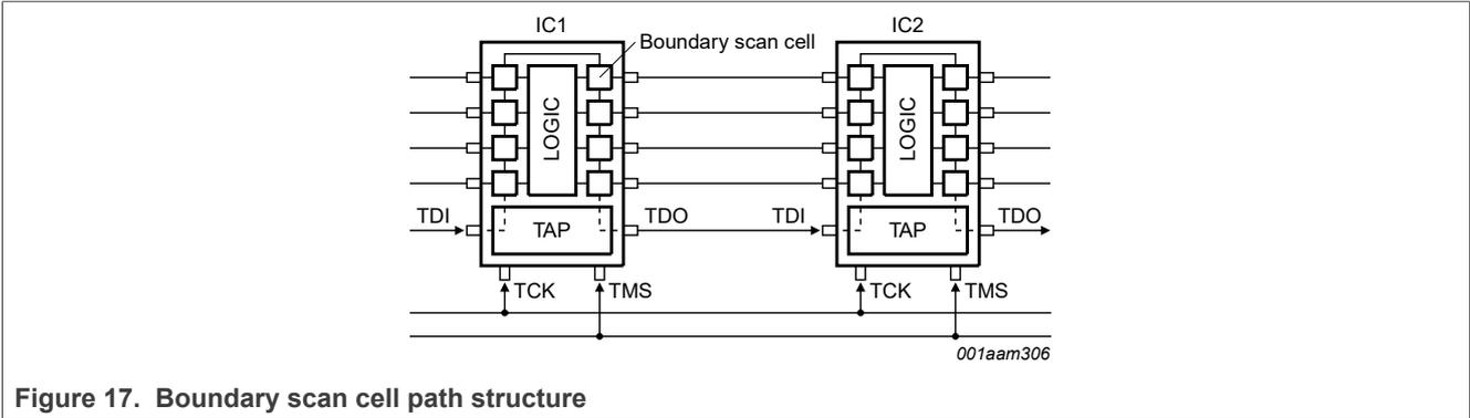
Figure 17. Boundary scan cell path structure
