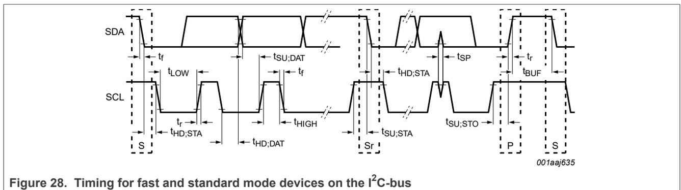
Figure 28. Timing for fast and standard mode devices on the I<sup>2</sup>C-bus
