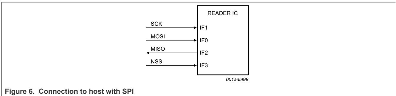
Figure 6. Connection to host with SPI
