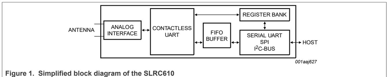
Figure 1. Simplified block diagram of the SLRC610
