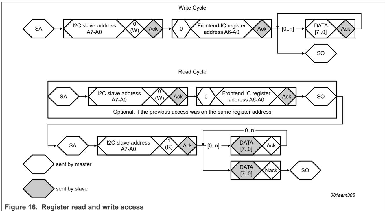
Figure 16. Register read and write access
