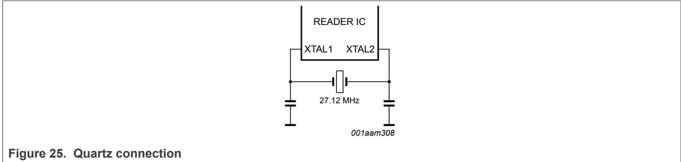
Figure 25. Quartz connection
