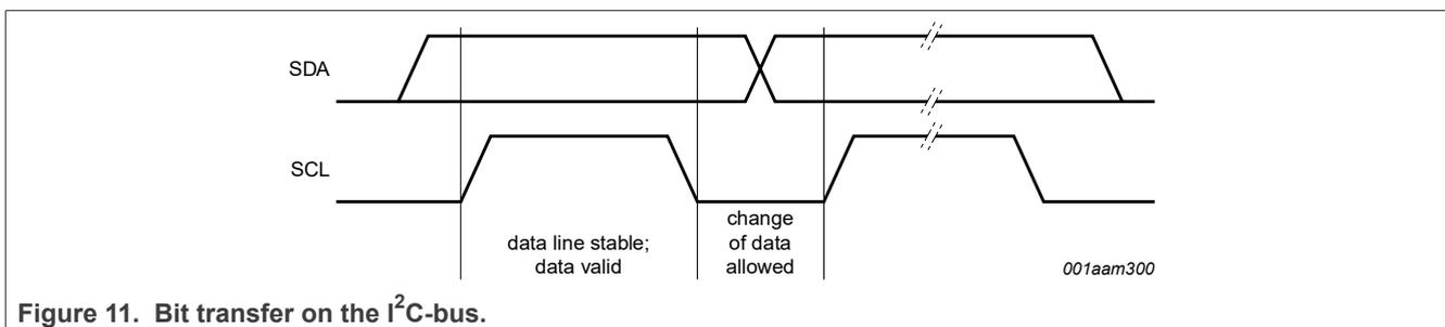
Figure 11. Bit transfer on the I<sup>2</sup>C-bus.
