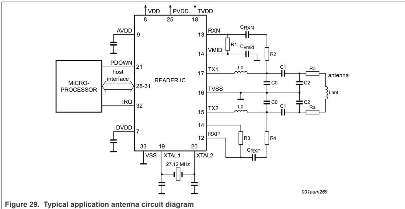
Figure 29. Typical application antenna circuit diagram
