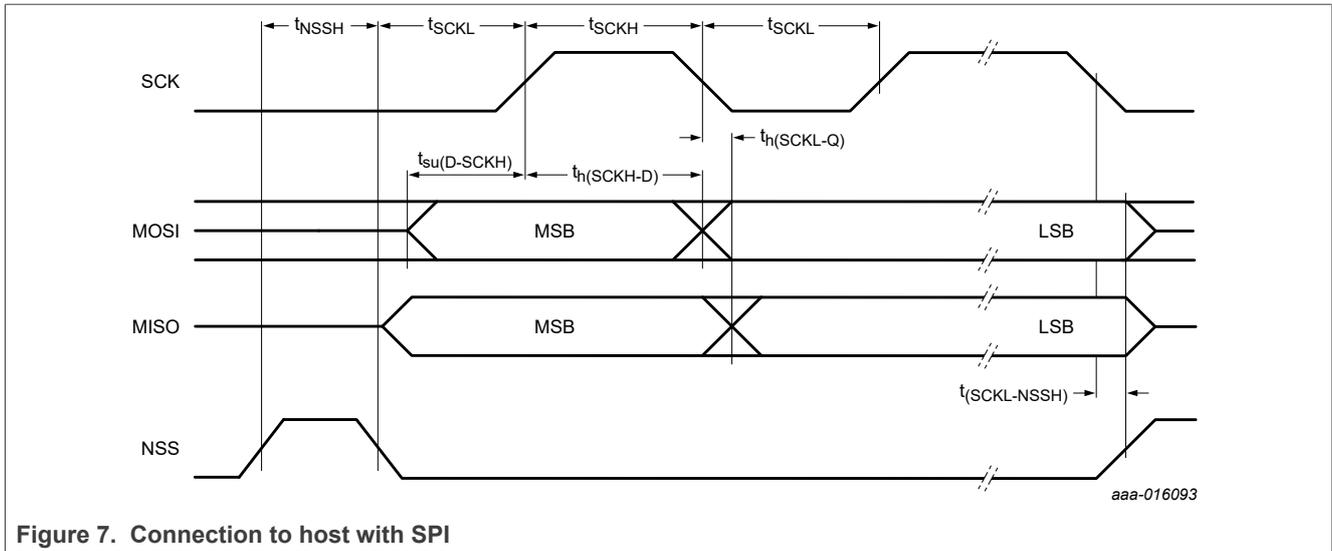
Figure 7. Connection to host with SPI
