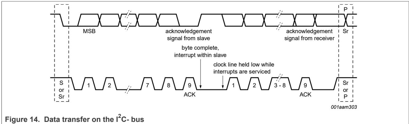
Figure 14. Data transfer on the I<sup>2</sup>C-bus
