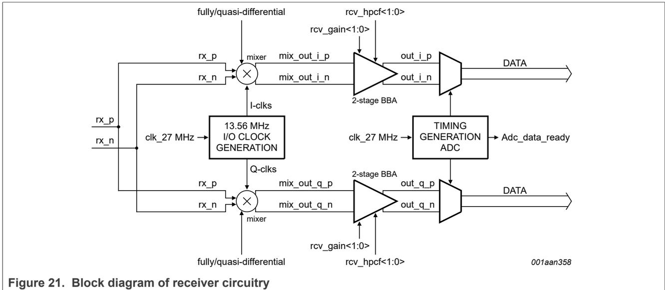
Figure 21. Block diagram of receiver circuitry
