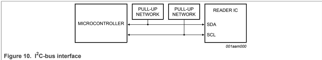
Figure 10. I<sup>2</sup>C-bus interface
