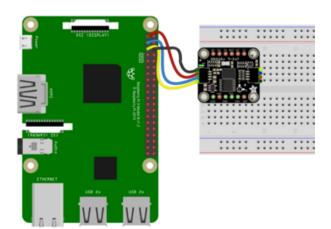
Pi 3V to sensor VCC (red wire)
