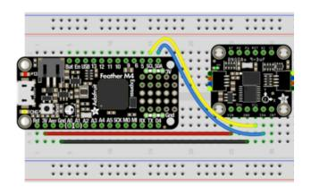
Board 3V to sensor VIN (red wire)
