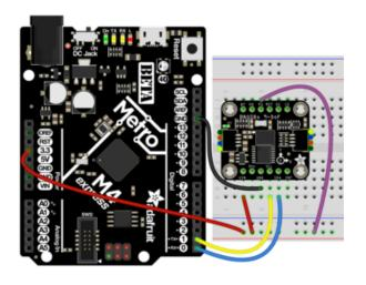
BNO085 Vin to the power supply, using the same logic level as your microcontroller. For the Metro M4 shown that is 3.3V, however check your board's documentation to be sure
