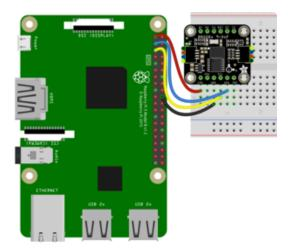
Pi 3V to sensor VCC (red wire)
