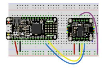
Board 3V to sensor VIN (red wire)
