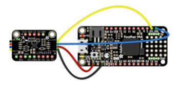
Board 3V to sensor VIN (red wire)
