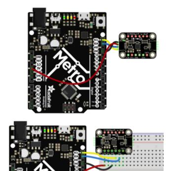
Connect board VIN (red wire) to Arduino 5V if you are running a 5V board Arduino (Uno, etc.). If your board is 3V, connect to that instead.
