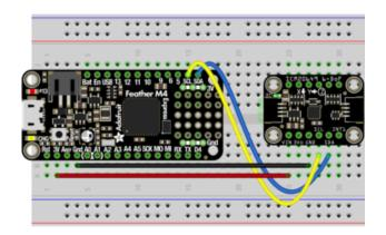
Board 3V to sensor VIN (red wire)
