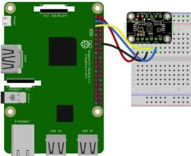
Pi 3V to sensor VCC (red wire)
