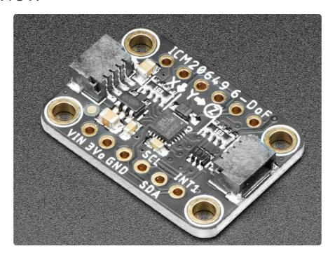
Most accelerometers have a similar range of measurements that they can make: often around 2G - 16G. Similarly most gyros can measure in the range of 250 degree/s to 2000 degrees/s. That's enough for many situations, however there are many situations where it's not quite enough. When measuring things like a golf swing, soccer ball kick or perhaps a fancy racing car, you need a bit more performance out of your motion sensor.
