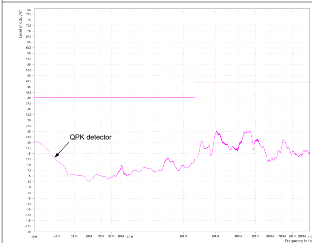
Figure 9-10. CISPR 32 Class B Radiated Emissions: Horizontal Polarization
