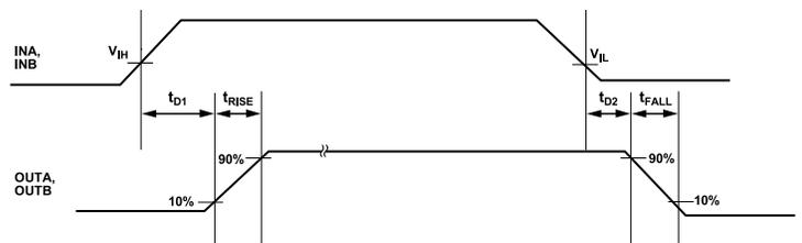
**Figure 2. Output Timing Diagram**
