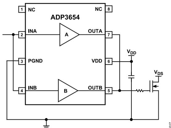
Figure 17. Parallel Operation
