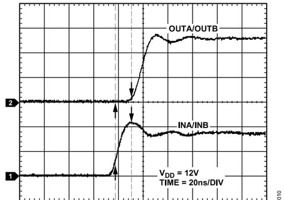
Figure 10. Typical Rise Propagation Delay
