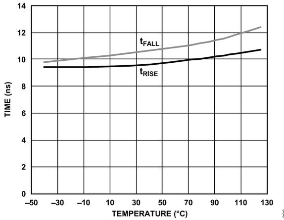
Figure 6. Rise and Fall Times vs. Temperature
