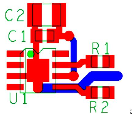
Figure 16. External Component Placement Example
