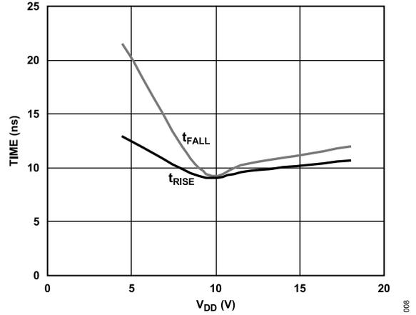
Figure 8. Rise and Fall Times vs.  $V_{DD}$
