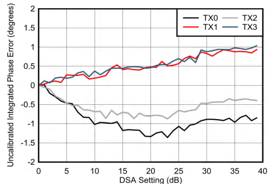
Figure 5-537. Uncalibrated Integrated Phase Error vs Channel at 7.1 GHz
