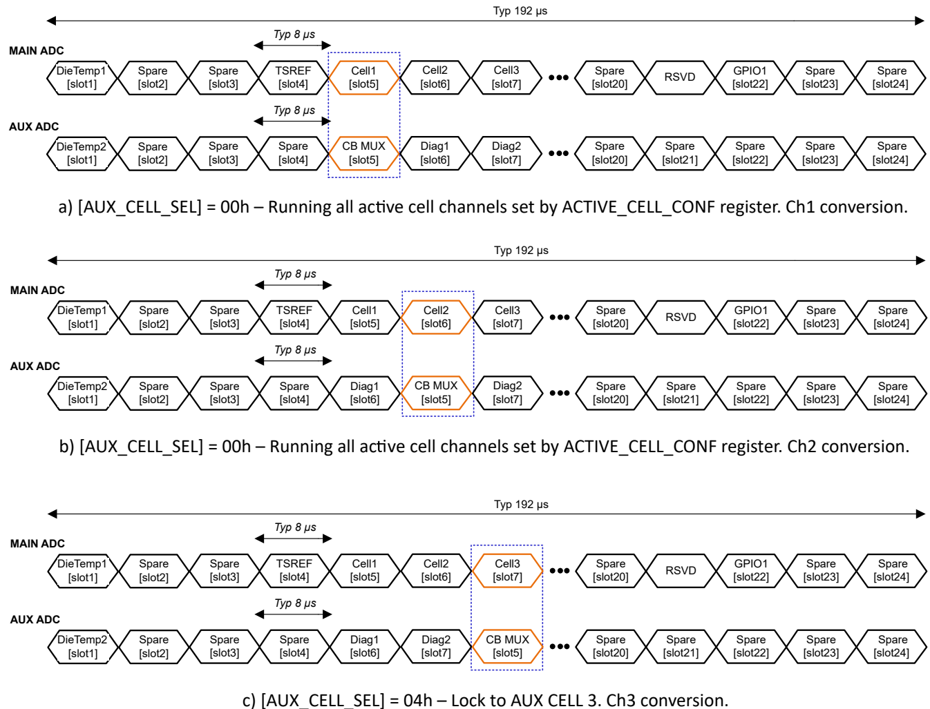
Figure 8-11. Synchronization Between MAIN and AUX ADC Sampling
