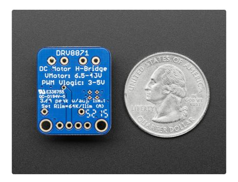
You can set the current limiting with an external resistor **Rlim**. We solder in a 30K resistor by default for a ~2A current limit, however you can remove this resistor and/or solder a resistor over it to change the resistance and change the limit.
