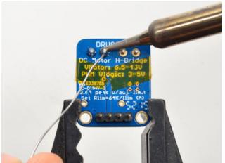
Solder in both pins of each terminal block. You can remove the tape when done.
