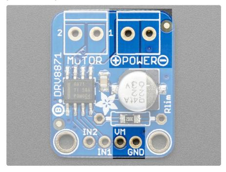
These two sets of pads are connected internally so you can use breadboard or terminal blocks to provide motor power. Use 6.5V-45VDC to power the motor and the chip. This isn't the same as the logic level of the chip, which is up to 5.5 VDC. You do not have to provide a logic level power supply to the chip, how nice is that?
