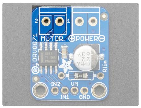
Pretty simple - this is where your motor goes! Works with any DC brushed motor. Use thick wires to avoid dropping voltage across the wire resistance
