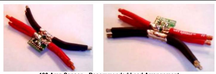
180 Amp Sensor – Recommended Lead Arrangement
