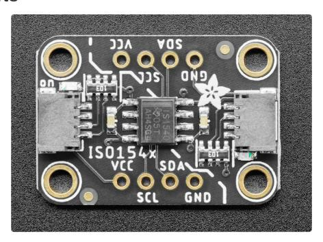
There are TWO SETS of power and data lines that are ELECTRICALLY ISOLATED! Each set is on one half of the isolation barrier.
