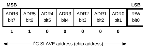
Figure 36. I 2 C Chip Address
