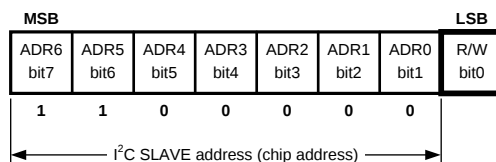
Figure 41. I 2 C Chip Address (see note above)
