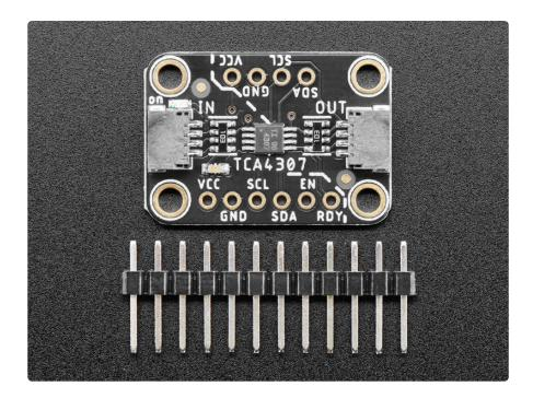
Usage is super simple. Connect the left side (IN) to your main board controller - Arduino, Raspberry Pi, Feather, etc. Then connect any I2C sensors you like to OUT side. Power is connected through - this isn't a power isolator, just a bus buffer. You can use 2.3 to 5.5V DC power and logic levels.
