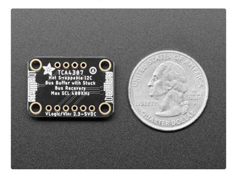
The chip can handle up to 400KHz I2C clock rates and even has stuck bus recovery: it automatically disconnects the bus if it detects either SDAOUT or SCLOUT are low for about 40 ms. Once the bus is disconnected, the device automatically generates up to 16 pulses on SCLOUT to attempt to reset the device which is holding the bus low.
