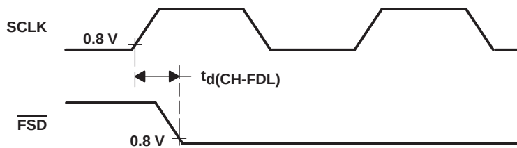
Figure 5–3. Master/Slave SCLK to \overline{\text{FSD}} Timing
