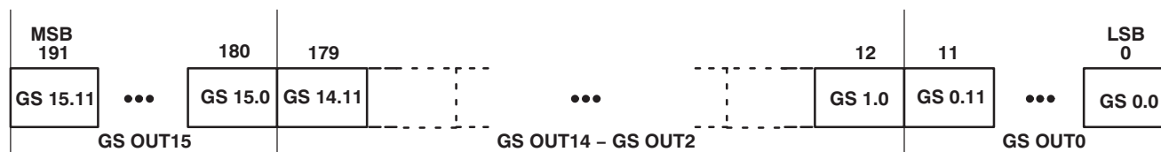
Figure 18. Grayscale Data Packet Format
