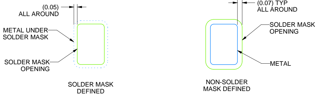
SOLDER MASK DETAIL
