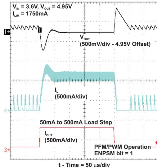
Figure 9. Load Transient
