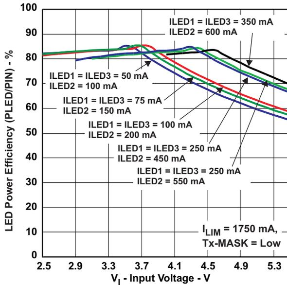
Figure 4. LED Power Efficiency vs Input Voltage
