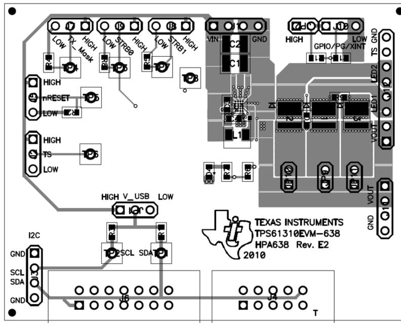
Figure 10. Assembly Layer
