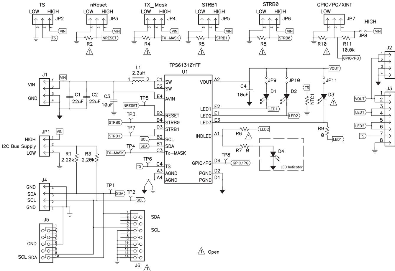
Figure 15. TPS61310EVM-638 Schematic
