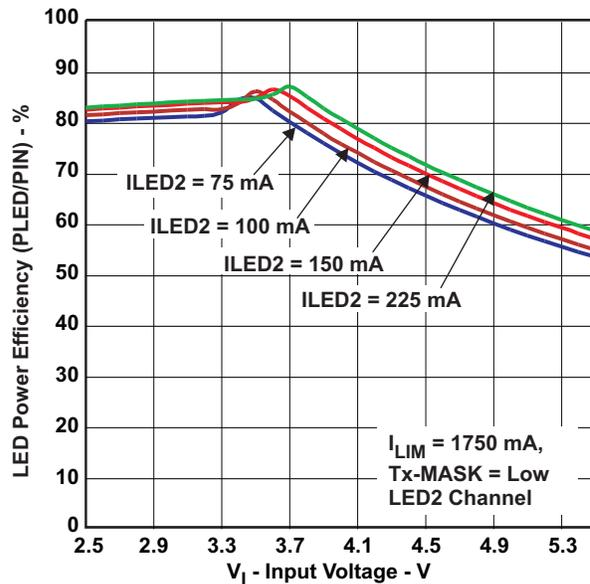
Figure 6. LED Power Efficiency vs Input Voltage
