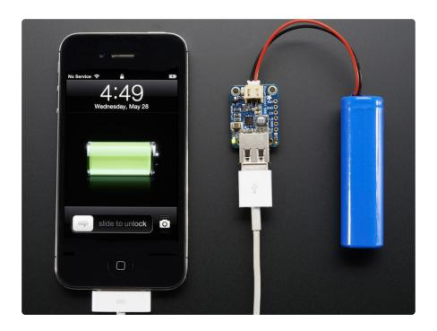
Great for powering your robot, Arduino project, single-board-computer such as Raspberry Pi or BeagleBone! Each order comes with one fully assembled and tested PCB and a loose USB A jack. If you are powering your project from USB, solder the USB A jack in (a 3-minute soldering task). If you would like to use a terminal block, pick up a 3.5mm 2pin block here (http://adafru.it/724) and solder to the output spot where the USB jack would go. Or dont solder anything in for a more compact power pack.
