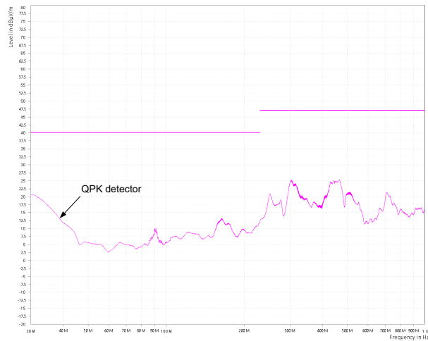
Figure 9-8. CISPR 32 Class B Radiated Emissions: Horizontal Polarization
