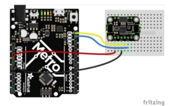
Board 5V to sensor VIN (red wire)
