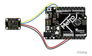
Board 5V to sensor VIN (red wire)
