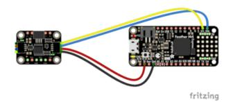
Board 3V to sensor VIN (red wire)
