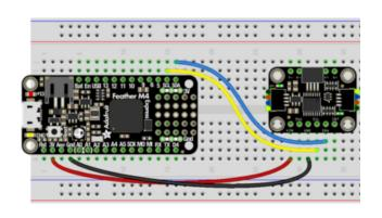
Board 3V to sensor VIN (red wire)
