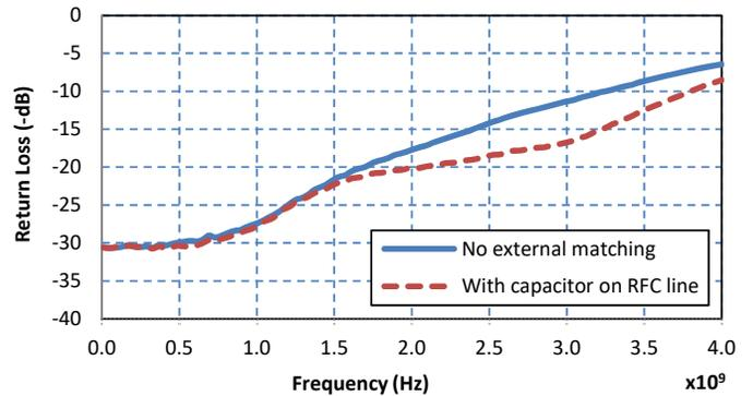
Figure 24. RFC Port Return Loss (RF1 Active)\*
