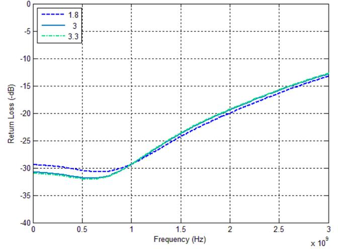
Figure 14. RFC Port Return Loss vs Temp (RF2 Active)\*
