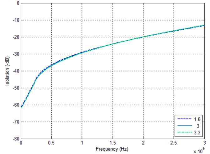
**Figure 10. RFX–RFX Isolation vs Temp**
