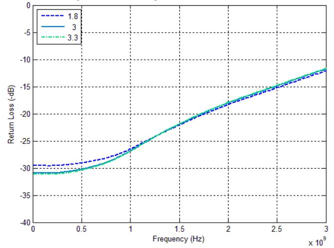
**Figure 18. Active Port Return Loss vs Temp (RF2 Active)\***
