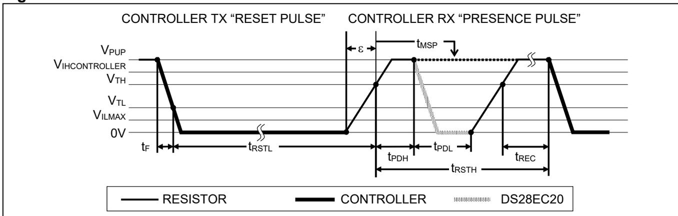
After the bus controller has released the line, it goes into Receive mode. Now the 1-Wire bus is pulled to  $V_{PUP}$  through the pullup resistor, or in case of a DS2482-x00 or DS2480B driver, by active circuitry. When the threshold  $V_{TH}$  is crossed, the DS28EC20 waits for  $t_{PDH}$  and then transmits a presence pulse by pulling the line low for  $t_{PDL}$ . To detect a presence pulse, the controller must test the logical state of the 1-Wire line at  $t_{MSP}$ .
