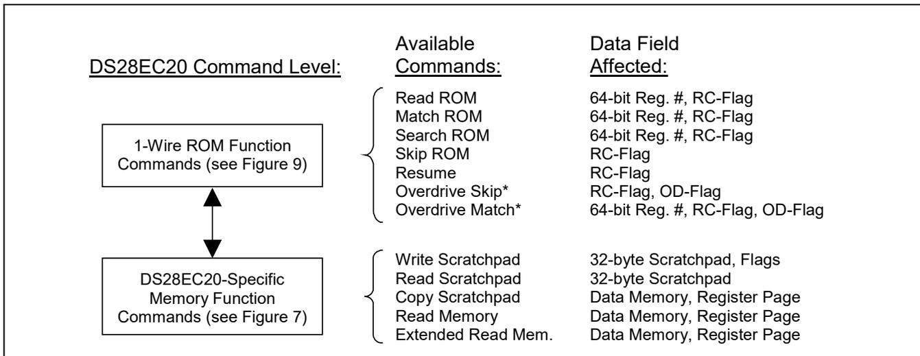
\* For operation at overdrive speed, the DS28EC20 requires  $V_{PUP}$  to be between 4V and 5.25V.
