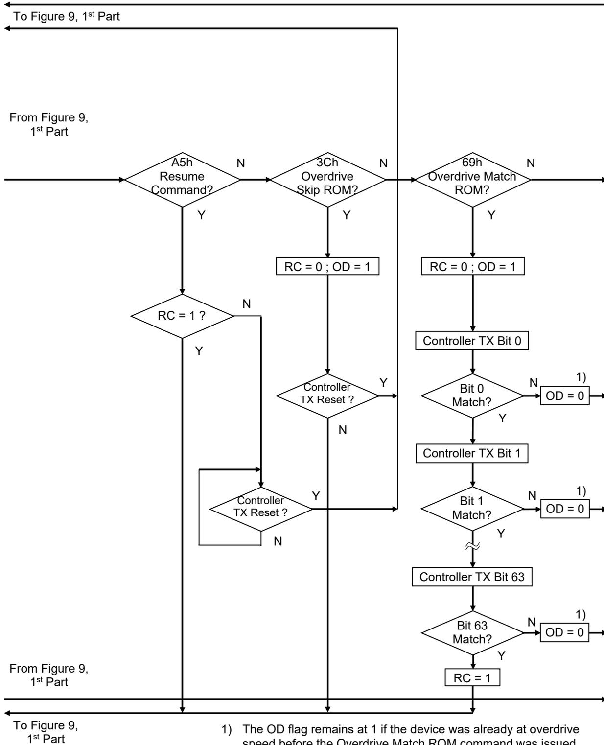
**NOTE:** For operation at overdrive speed, the DS28EC20 requires  $V_{PUP}$  to be between 4V and 5.25V.
